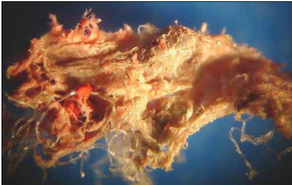
Photograph 11 Red particle embedded in fused matrix of rope filaments
