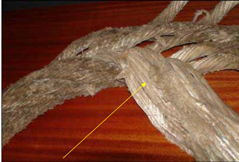
Severe damage to cluster of core rope yarns
