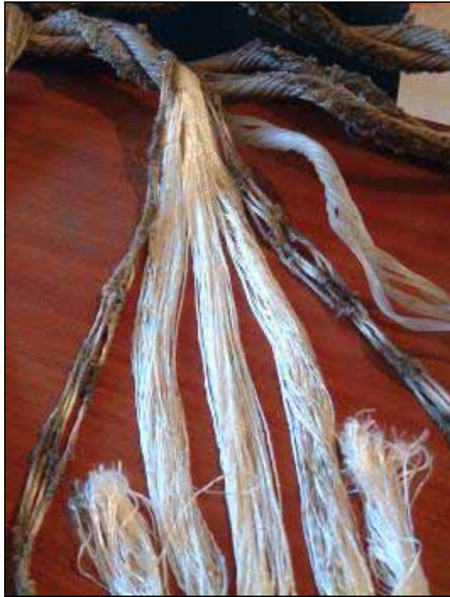
Photograph 15 Strand from 'clear' sample, unraveled to core reveal textile yarns
