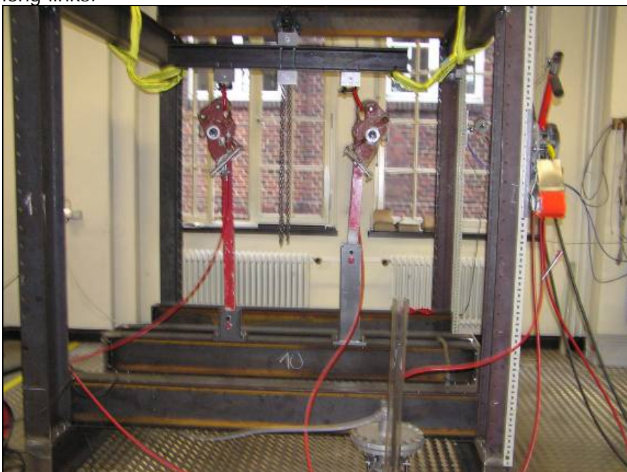
Figure 9: Test Arrangement: Test foundation structure with hoisting hooks, release cables, hydrostatic pressure cell und central release unit. Release cables are directed on top of foundation structure with generous radius between the elements.
