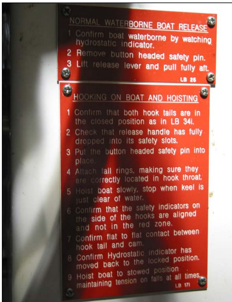
Figure 29: Operating plate LB 25 and operating plate LB 171.
