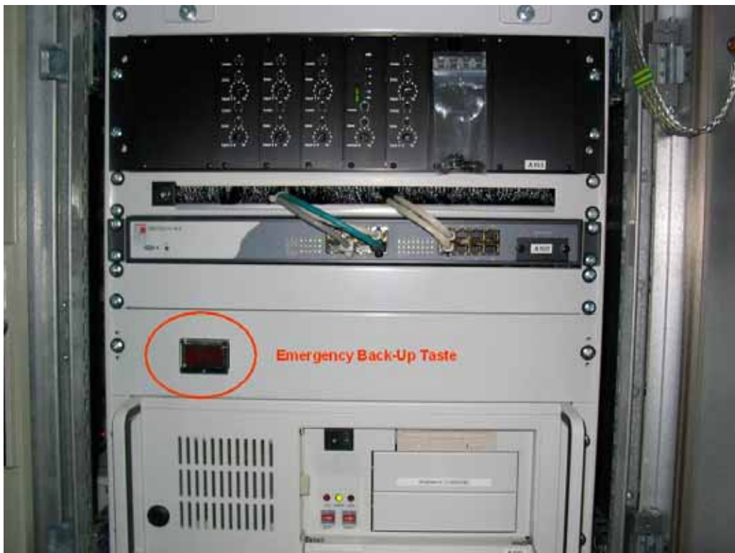
Abbildung 7: Emergency-Back-Up-Taste am VDR (Foto: BSU)
