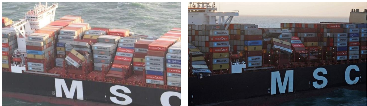
Figure 4-42: Loss of containers on the wave (port) side of the MSC Zoe, in the area where during the model tests the largest number of green water events was observed (view for port side).
