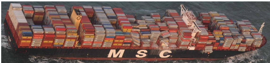
Figure 4-41: Spatial distribution of green water events as observed during three tests at zero speed, compared with the damaged container stacks of the MSC Zoe (view from starboard side).
