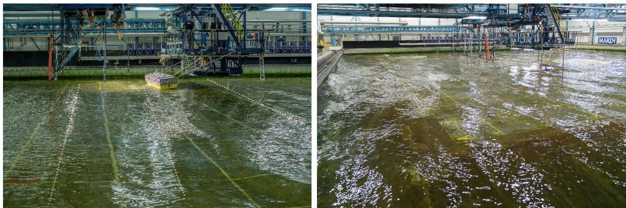
Figure 2-3: Long-crested waves (left) and short-crested waves (right) The dash lines underline the crest of the long-crested waves.
