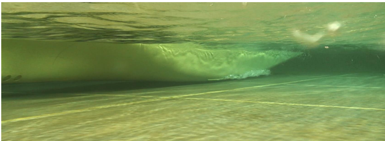
Figure 4-35: Still of underwater footage ( t=339 \text{ s} ), H_s = 6.5 \text{ m} , T_p = 14.5 \text{ s} , short-crested waves, V_s = 10 \text{ kn} .
