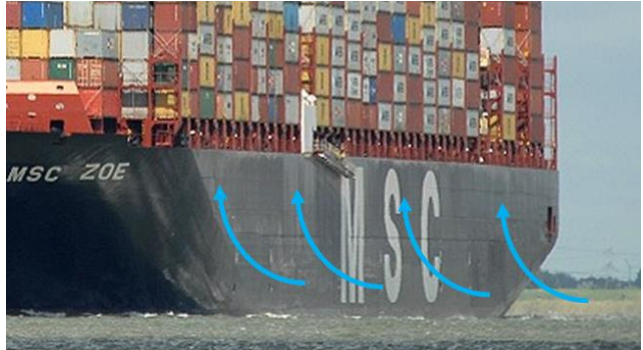
Figure 4-38: Shallow, steep waves can reflect strongly against the side of the ship, resulting on 'green water' reaching the deck and the containers.
