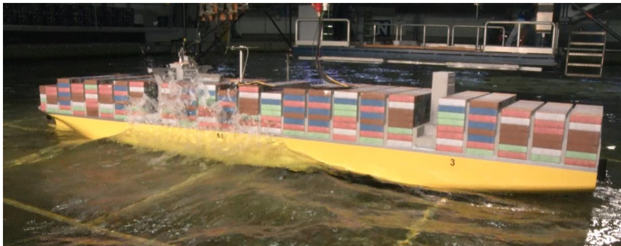
Figure 4-45: Occurrence of wave-induced slamming (along with green water) on the side ( t=11005 s) H_s = 6.5 m, T_p = 14.5 s, short-crested waves, V_s = 0 kn, water depth 21.3 m.
