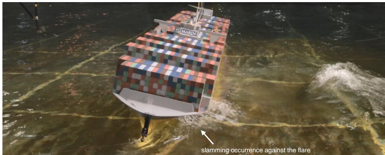
Figure 4-43: Occurrence of wave-induced slamming on the bow flare ( t=6440 s) H_s = 6.5 m, T_p = 14.5 s, Short-crested waves, V_s = 0 kn, water depth 21.3 m.
