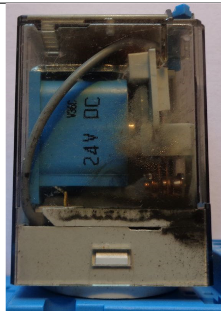
Picture 4: Dust or smut in STBD relay
