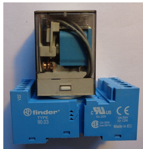
Picture 2: One of the relays with socket
