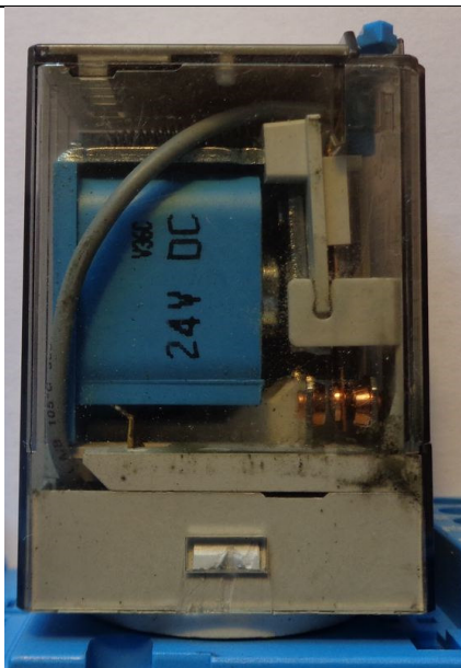
Picture 3: Dust or smut in PORT-relay
