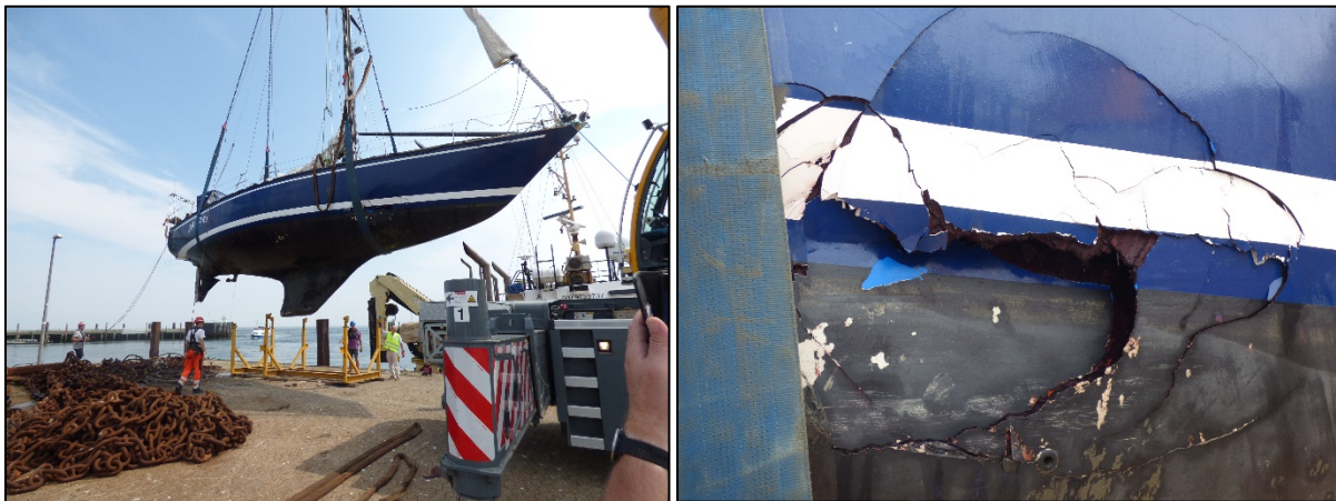
Figures 14 and 15: Salvage of the SHARKY with penetrated hull 16
