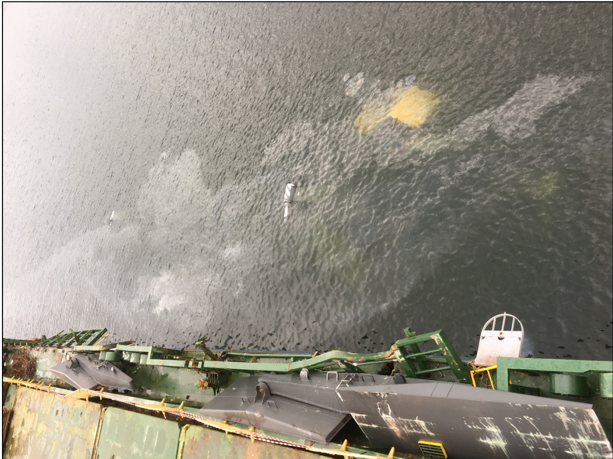
Figure 10: The cranes are submerged. Escaping oil and damage to the vessel are visible. 12
