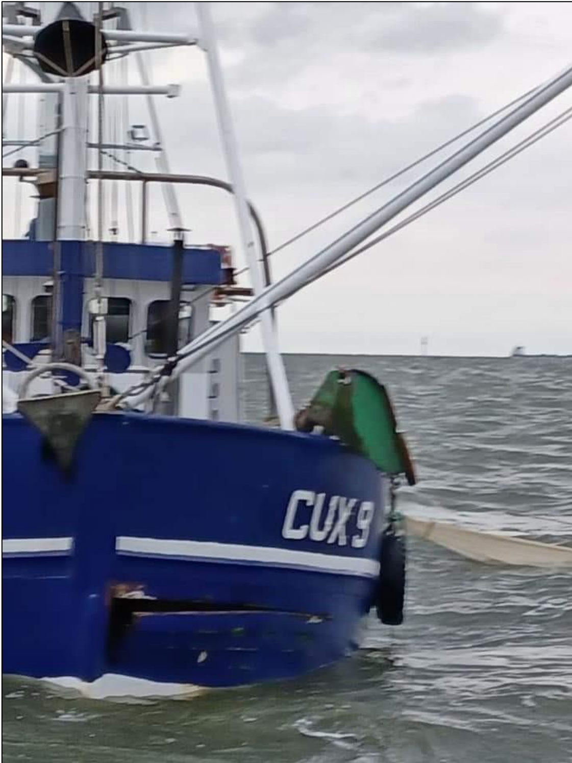
Figure 14: Loose planks at the bow of the RAMONA 21
