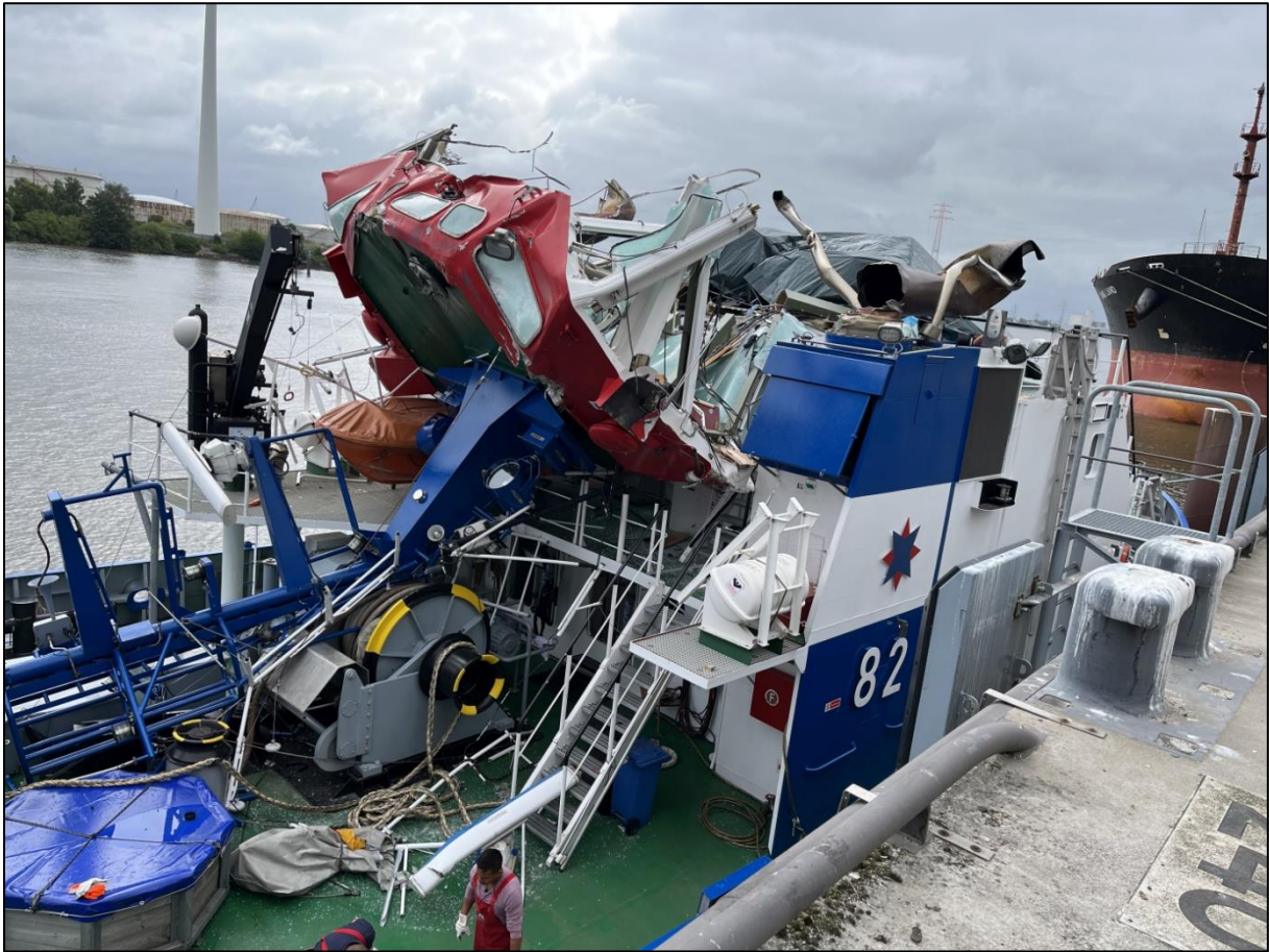
Figure 15: The heavily damaged FAIRPLAY 82 after the collision 24
