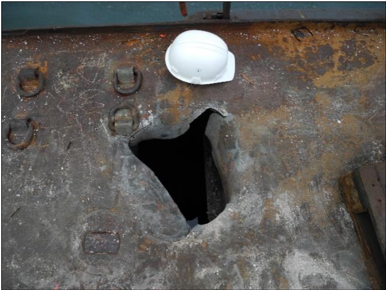
Figure 20: Hole in the MERI's deck together with a helmet for size comparison 29
