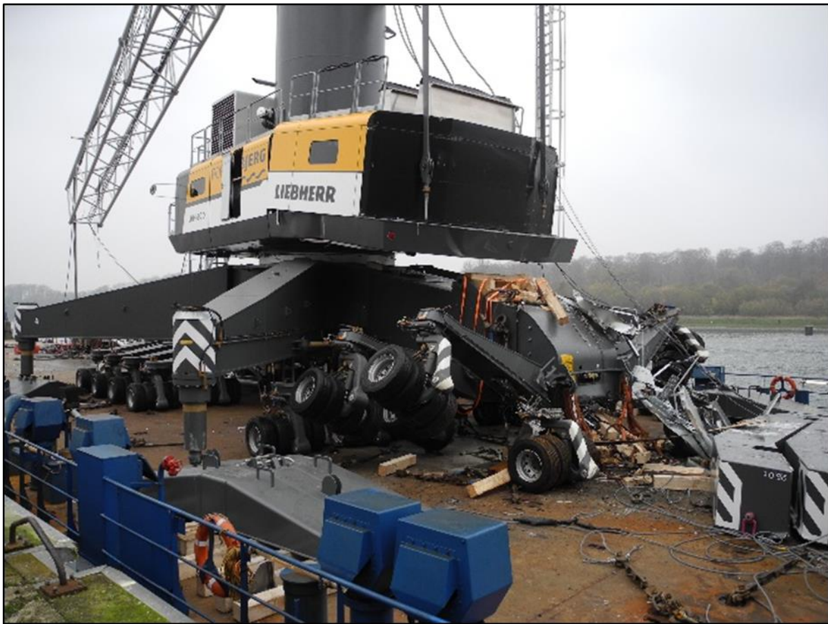
Figure 19: The damaged crane 28
