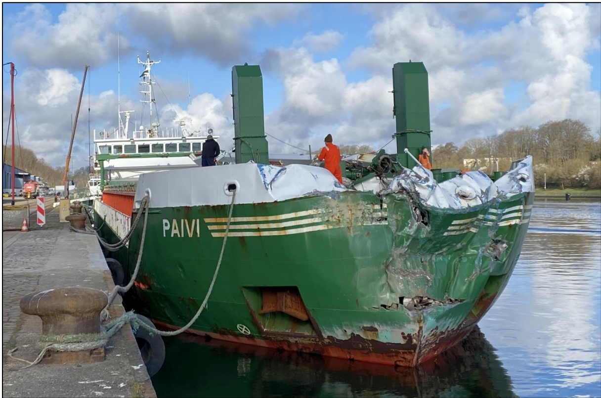
Figure 6: The deformed bow of the PAIVI 14
