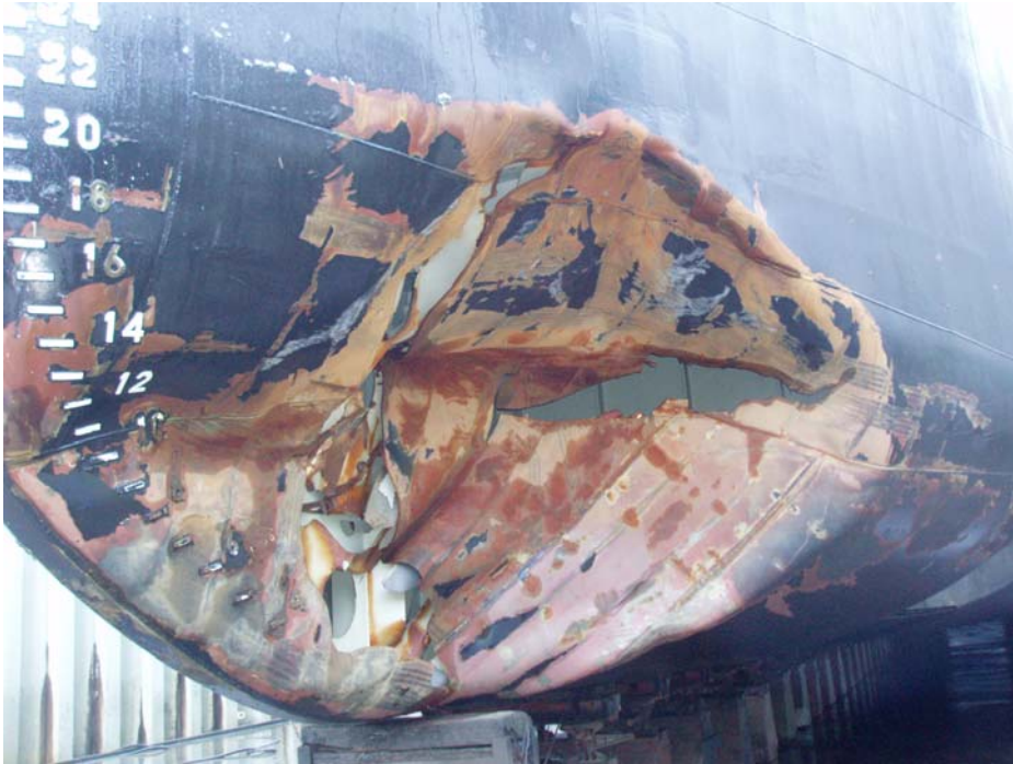
Bottom damage after collision
