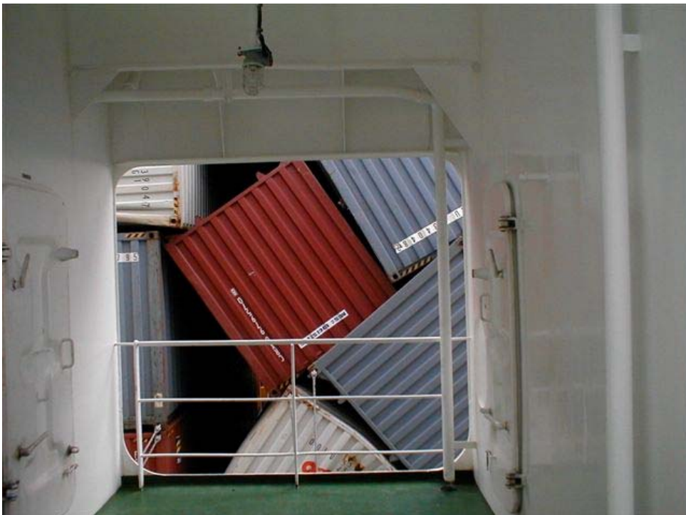
Loss overboard of containers and damage caused by containers
