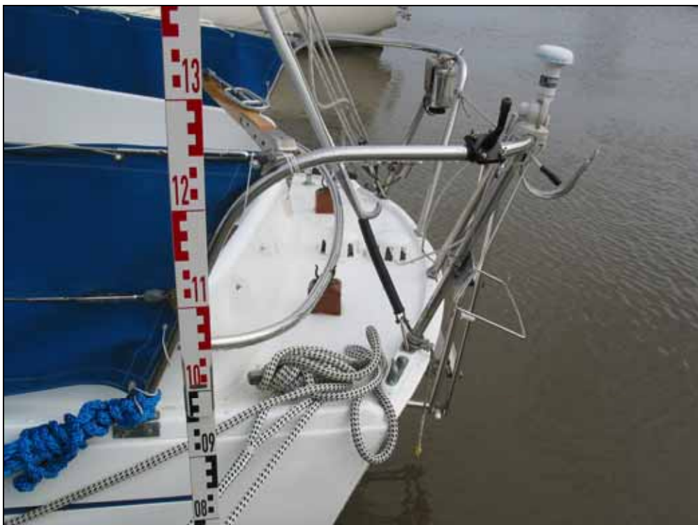
Figure 1: Determination of freeboard and rail height on a leisure craft
