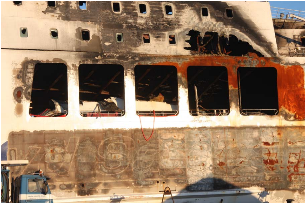
Fire on the ro-ro passenger vessel LISCO GLORIA, BSU Investigation Ref.: 445/10, published on 01/02/2012 Source: BSU
