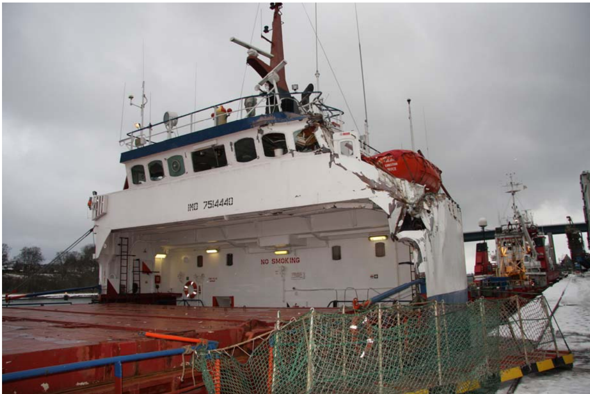
Destroyed bridge of the general cargo vessel MALAGA after a collision with the container vessel NATIONAL GLORY, BSU Investigation Report Ref.: 523/10, published on 12/12/2011 Source: BSU
