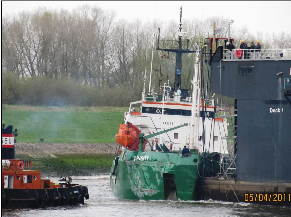
Fore section of the ZAPADNY Y wedged into the front end of the floating dock
