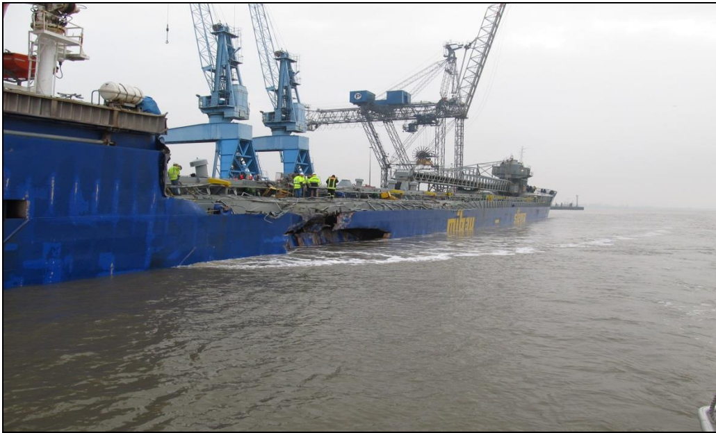
Water ingress on the starboard side of the bulk carrier SPLITTNES; BSU investigation ref. 507/11, investigation ongoing at 31 December 2012
