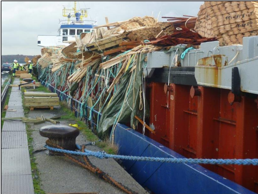
Shifted cargo on the ROSEBURG 3
