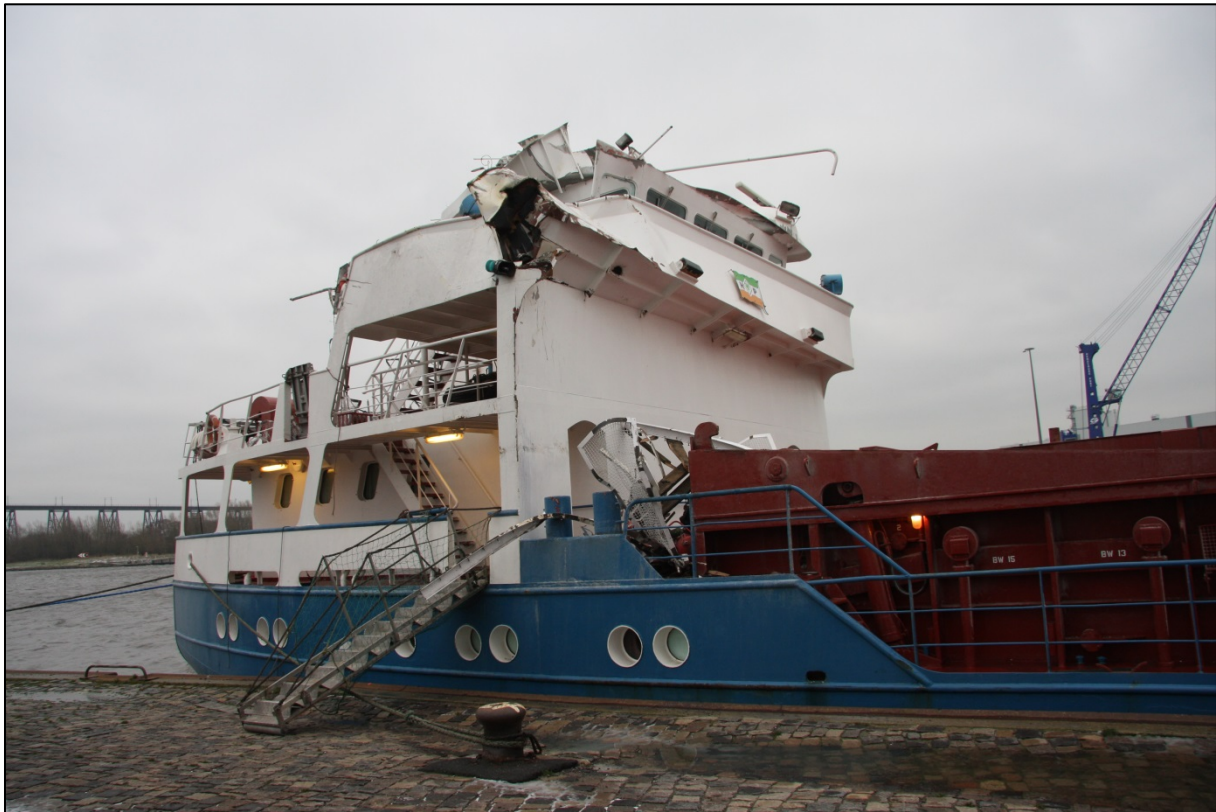
Damage to the EVERT PRAHM
