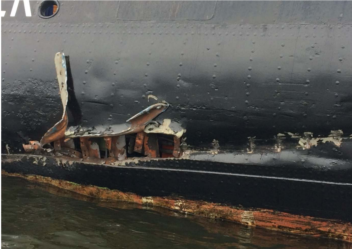
Torn shell plating on the STETTIN (source: WSP)
