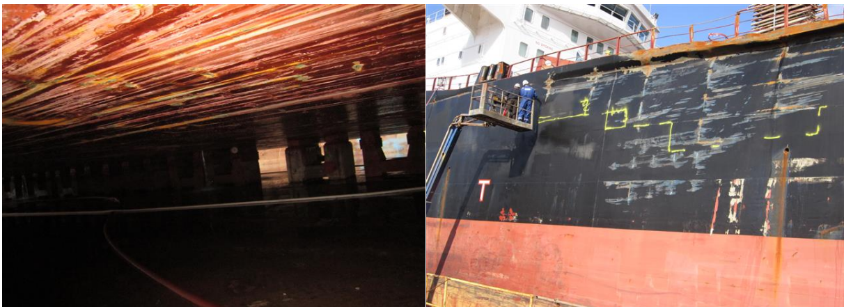
Damage to the SEATROUT (left figure: deep scratches on the underwater hull; right figure: dents and abrasion marks on the starboard side (source: BSU))
