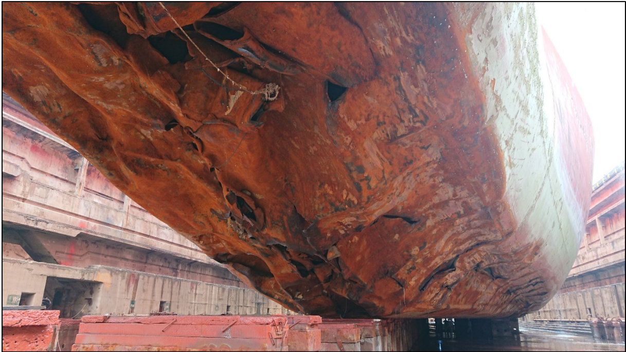
Heavy damage to the underwater hull found in the shipyard. Source: Owner
