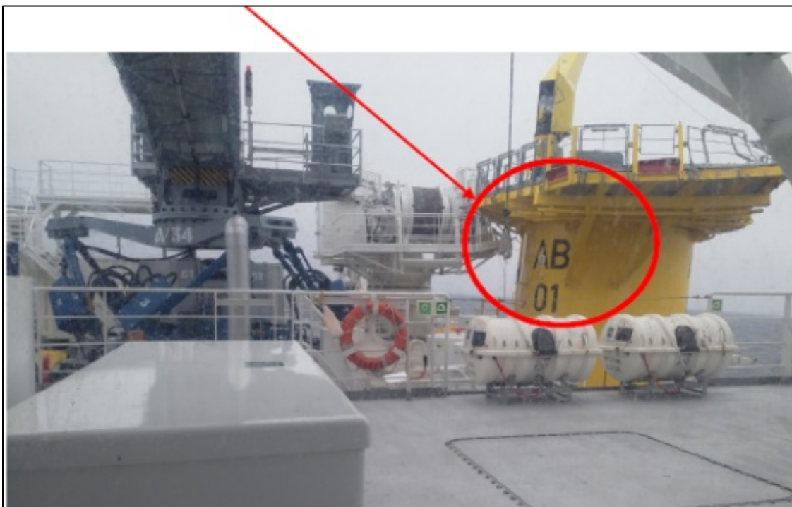
Second allision: The loading crane rammed the platform. Source: VBMS
