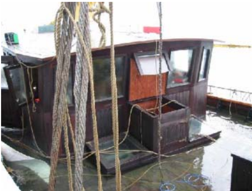
Photo 19, Skylight fore edge of wheelhouse, closed
