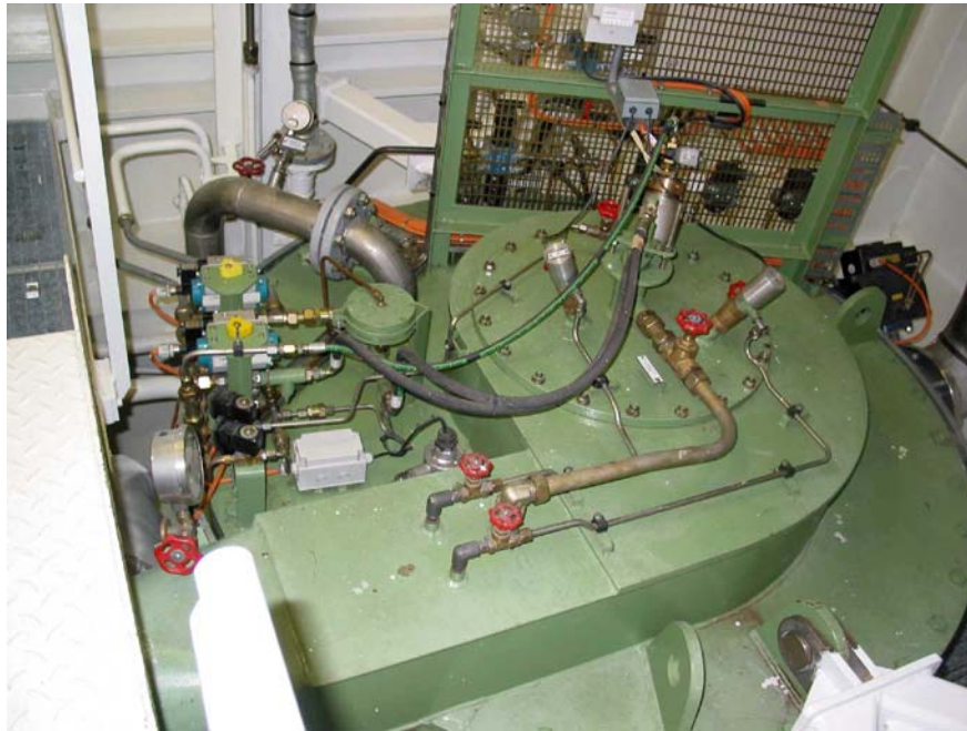
Figure 9: I.G. top with lid for combustion chamber
