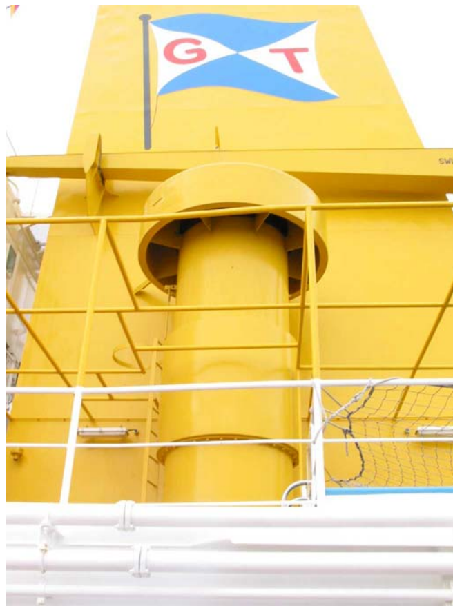
Figure 14: Portside engine room ventilator
