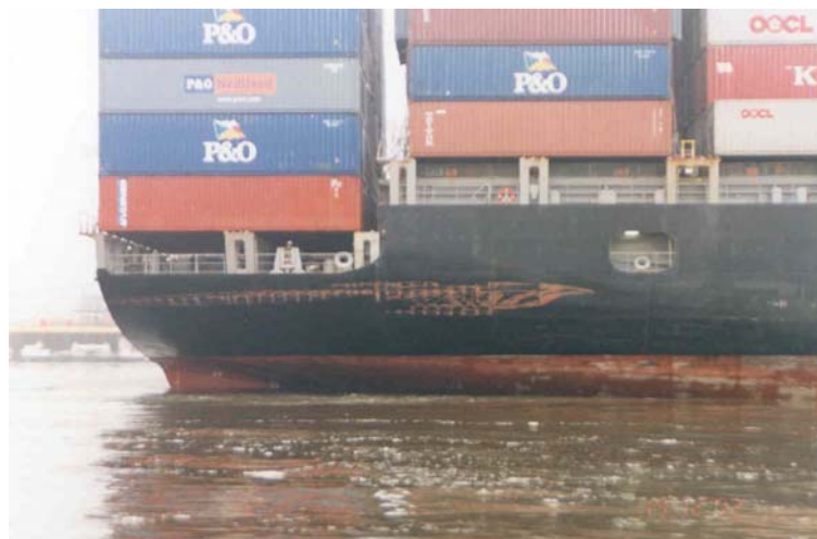
Figure 5: Damage to CMV P&O NEDLLOYD GENOA, starboard side, aft ship 1
