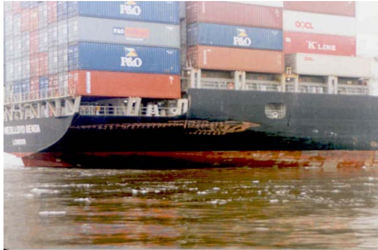
Figure 6: Damage to CMV P&O NEDLLOYD GENOA, starboard side aft ship 2
