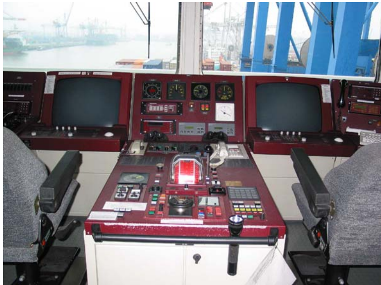
Figure 4: Control console looking at the radar sets
