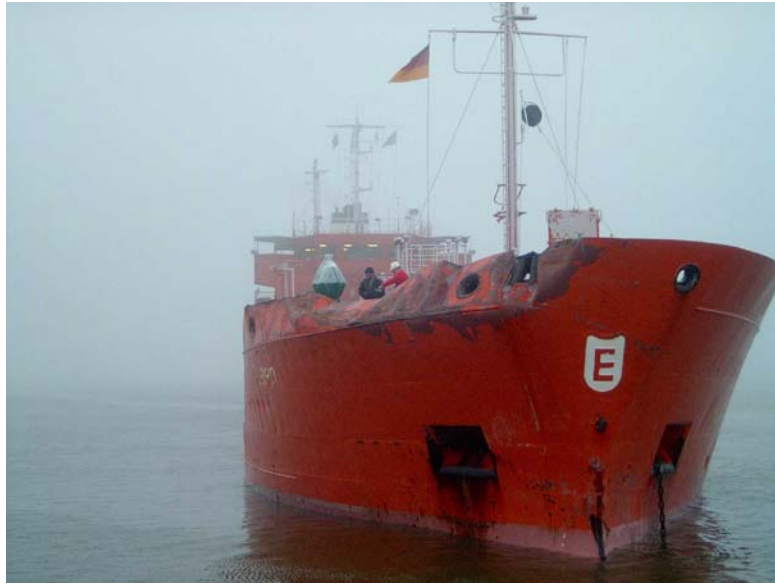
Figure 7: Damage to MT EBRO, foreship
