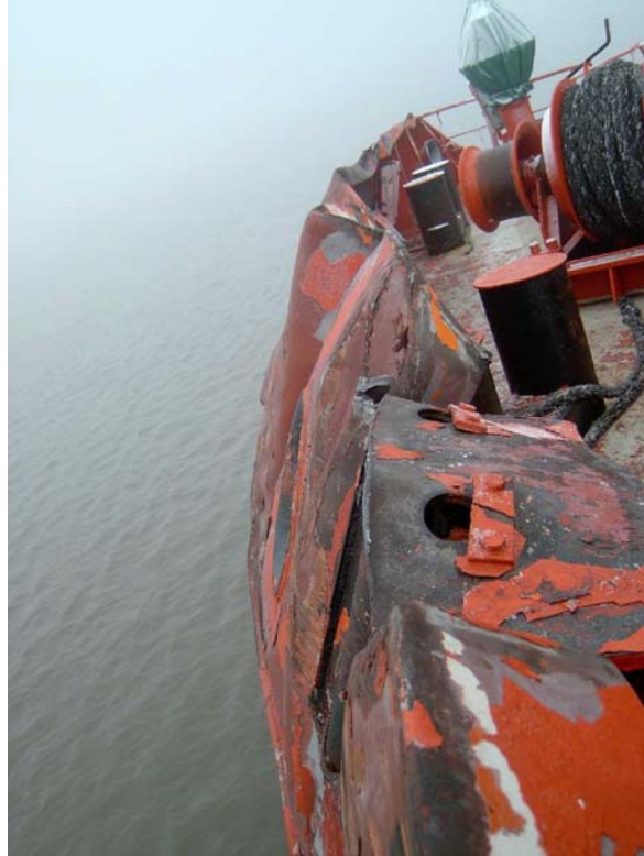
Figure 9: MT EBRO, deformed bulwark
