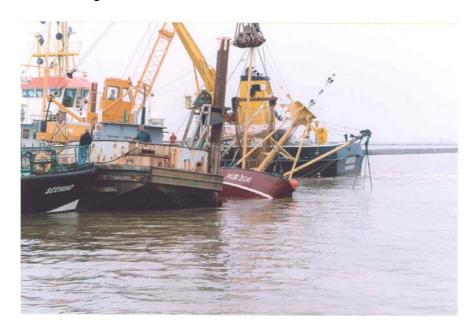
In the second salvage attempt the rescue cruiser BERNHARD GRUBEN and the Buoy Layer NORDEN pulled the foundered cutter approx. 250 m through the mud to the Muschel Pier. After this the cutter was lifted so far out of the water by a shore-based crane that the open apertures through which water flowed were above the water level. The cutter was then freed from mud and water using drain pumps.
