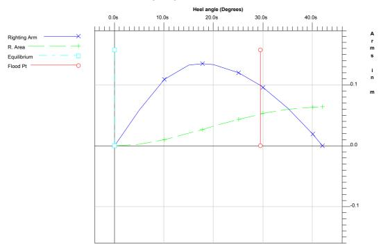
In particular in this calculated stability case the range of stability is only 43.41° (60° required), the righting arm at 30° is only 0.108 m (0.20 m required), and the areas below the righting arm curve from 0° to 40° and from 30° to 40° are not sufficient either.
