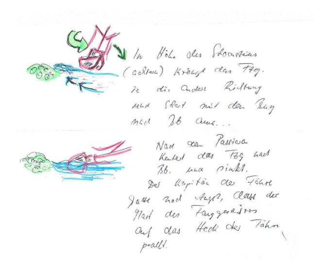
On a level with the stack (aft) the vessel lists in the other direction and the bow veers to port.
