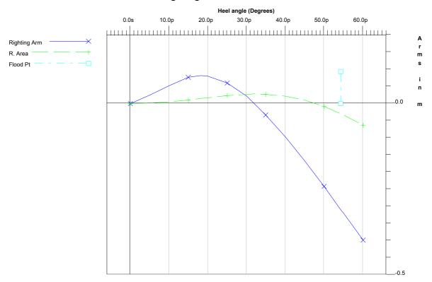
The GM is 0.269 m (required 0.35 m), the range of stability in this case is only 32°, the righting arm at 30° is 0.02 m, and the areas beneath the righting arm curve are absolutely insufficient.
