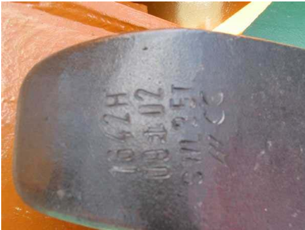
Figure 10: Certified fairlead shackle, Tug AXEL
