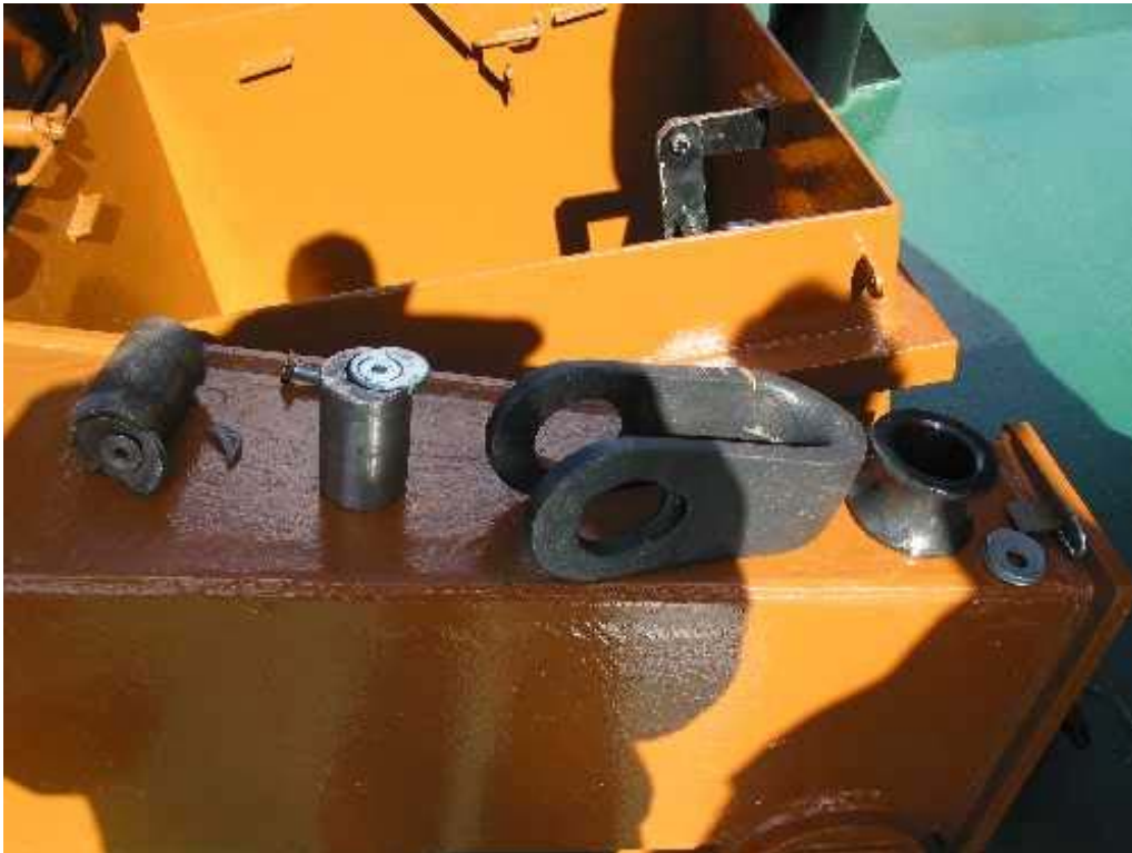
Figure 7: Fairlead-Shackle 90M new with damaged bolt
