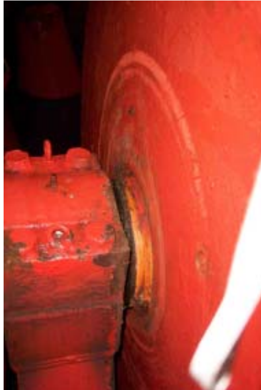
Figure 4: Grinding/abrasion traces on the side plate (Photo Criminal Investigation Department Bremerhaven)
