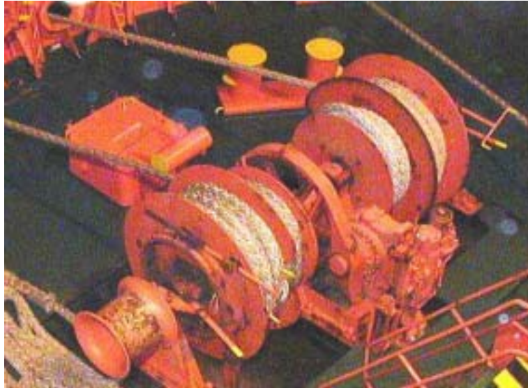
Figure 15: Midships winch, 11 November 2003 (Photo River Police Bremerhaven)
