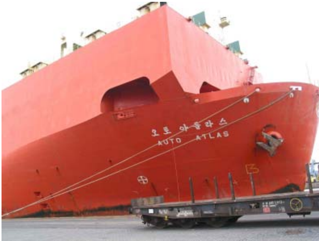
Figure 19: Bow spring beneath the forecastle superstructure
