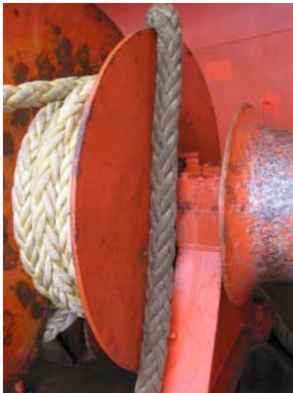
Figure 12: Reconstruction of the line clamp according to testimony of Boatswain on 5 February 2004
