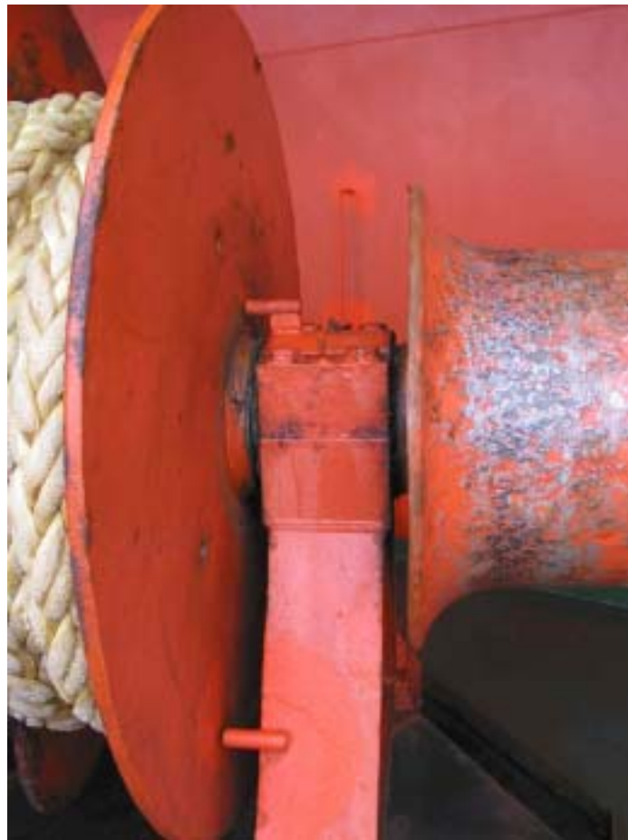
Figure 22: Deflector welded on
