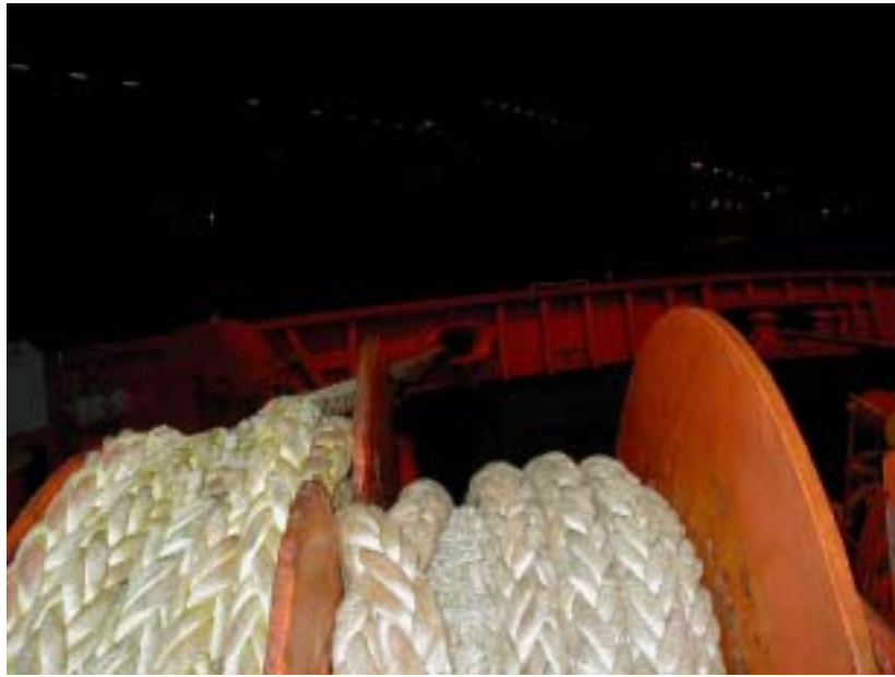
Figure 20: Rope in the working part of the winch under load and exceeding the proposed rope layers
