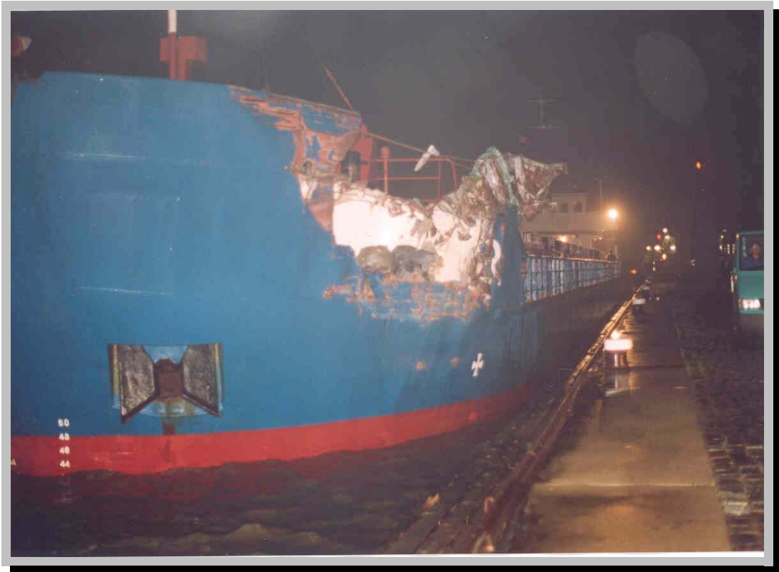
Figure 6: Photo of damage 1 MV BOUNDER
