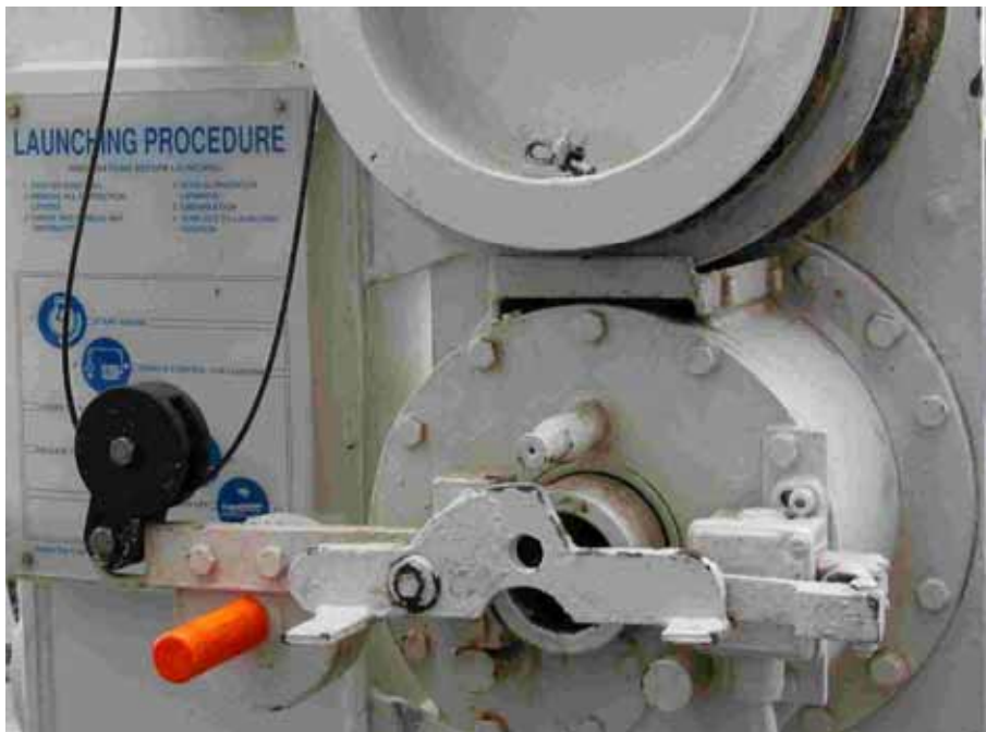
Figure 6: Safety bar locked
