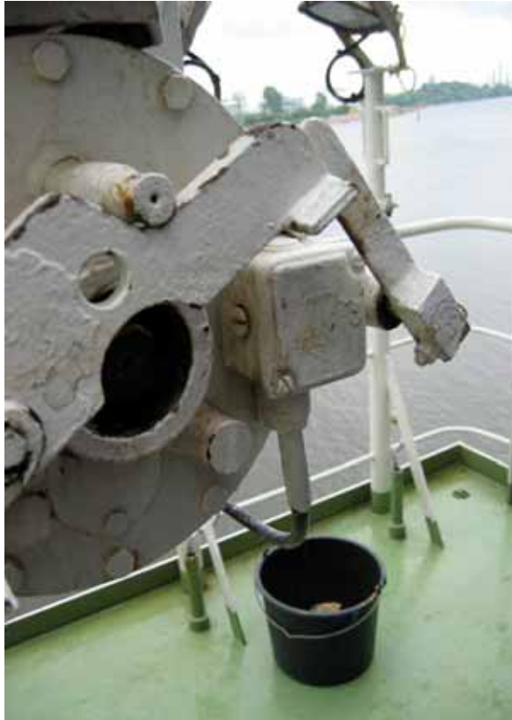
Figure 15: Limit switch, end position
