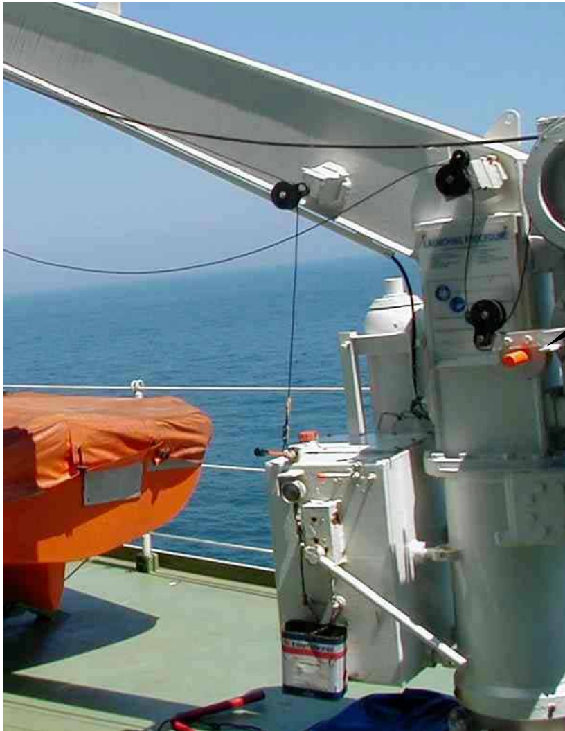
Figure 21: Mounted safety bar shortly after the accident
