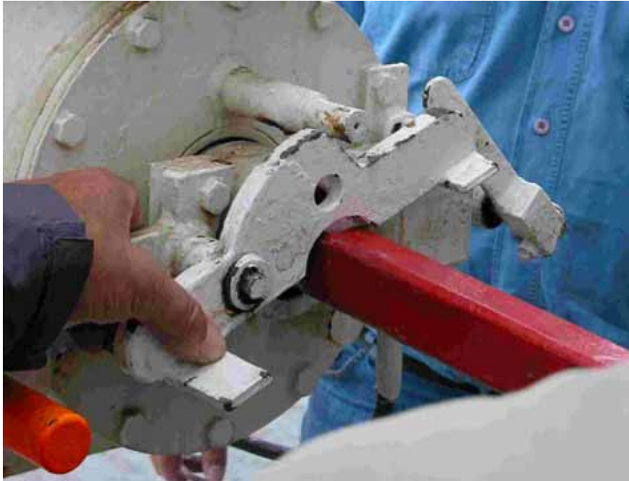
Figure 7: Safety bar opened (crank-handle in place)
