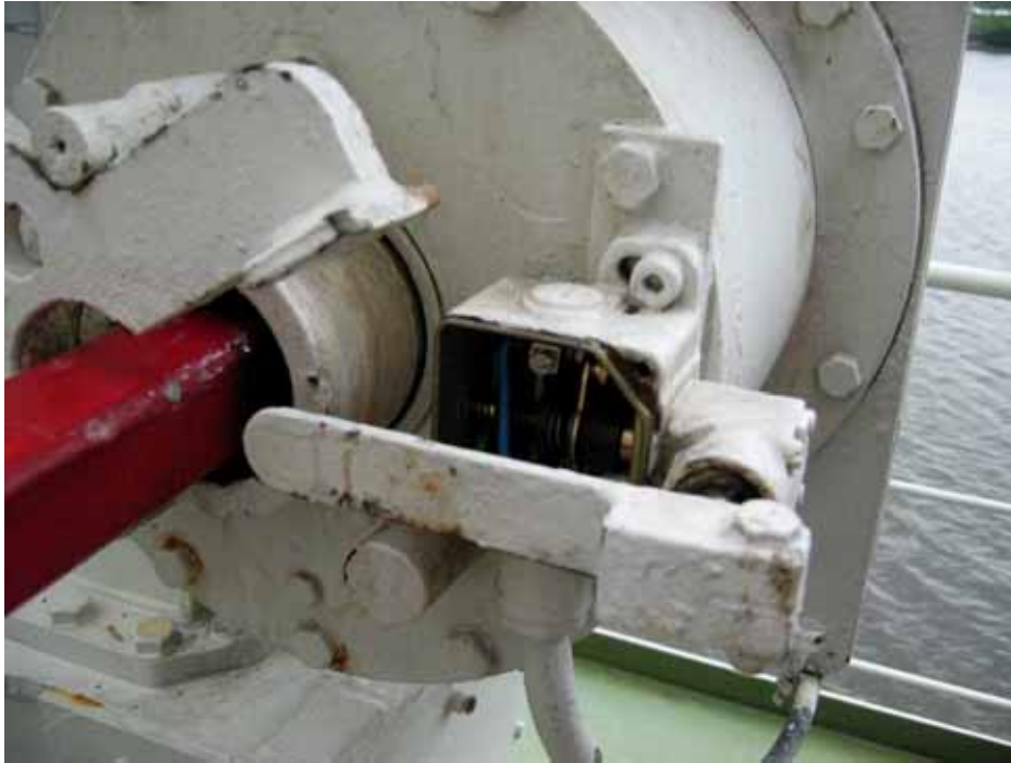
Figure 20: Limit switch lever beneath the safety bar (crank-handle in place)
