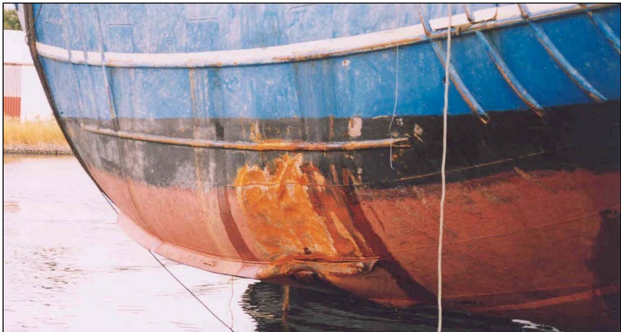
Figure 14: Photo of damage 4 – FV GRETJE GRE8
