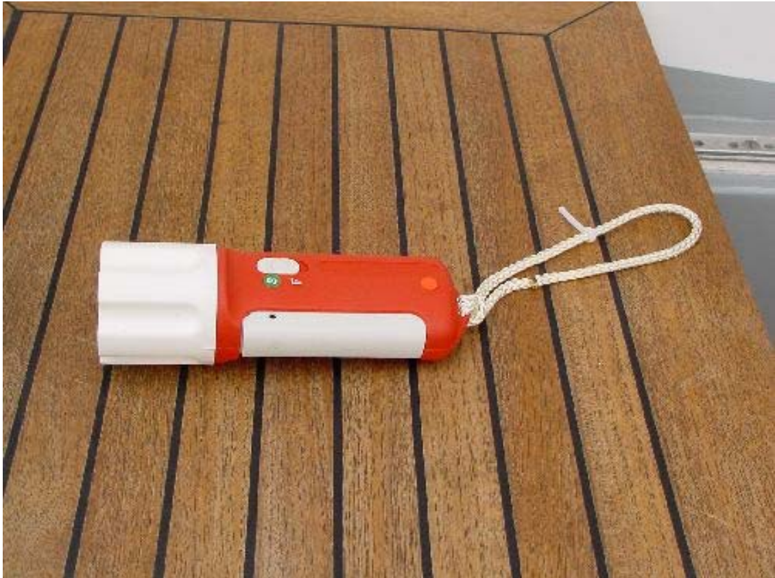
Figure 9: Distress signal unit
