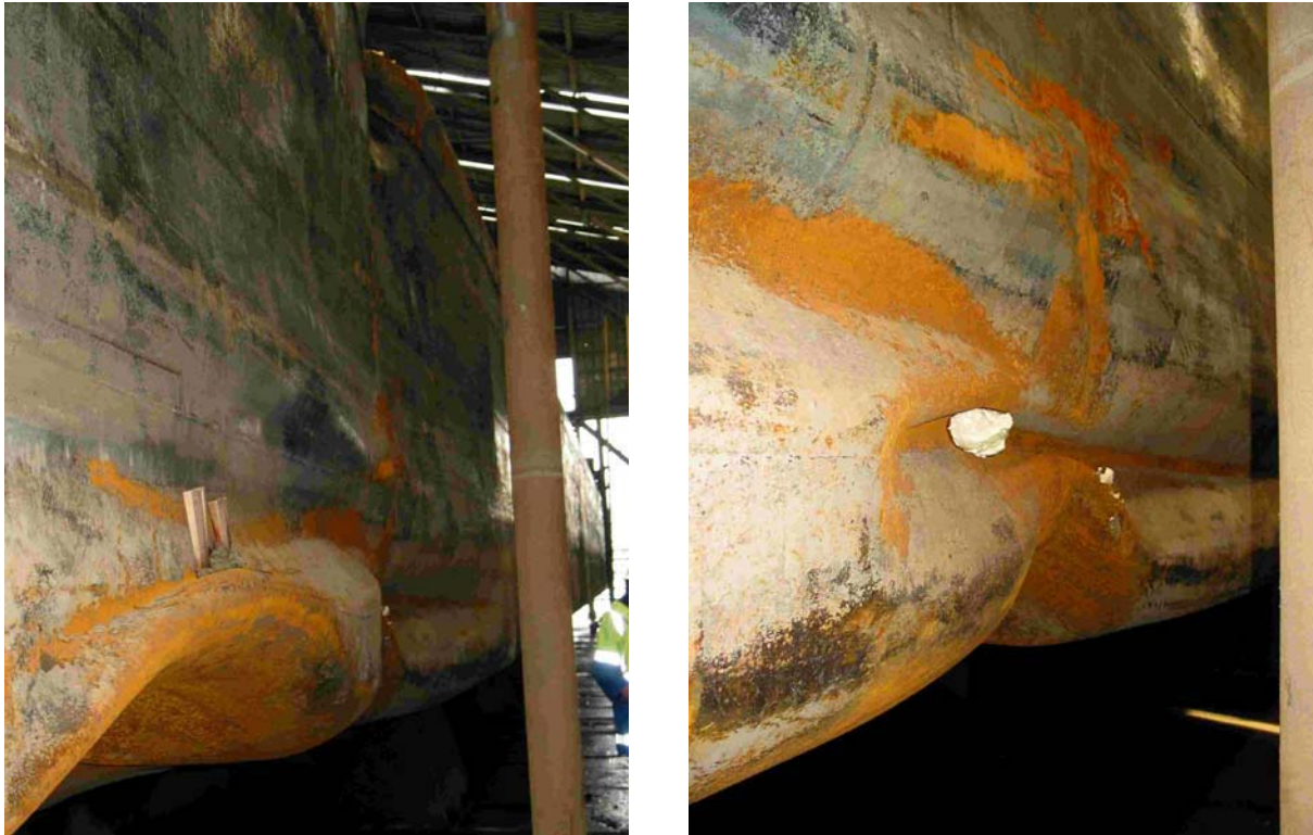
Figure 12: Deformation and cracking in the outer plating of ENA 2
