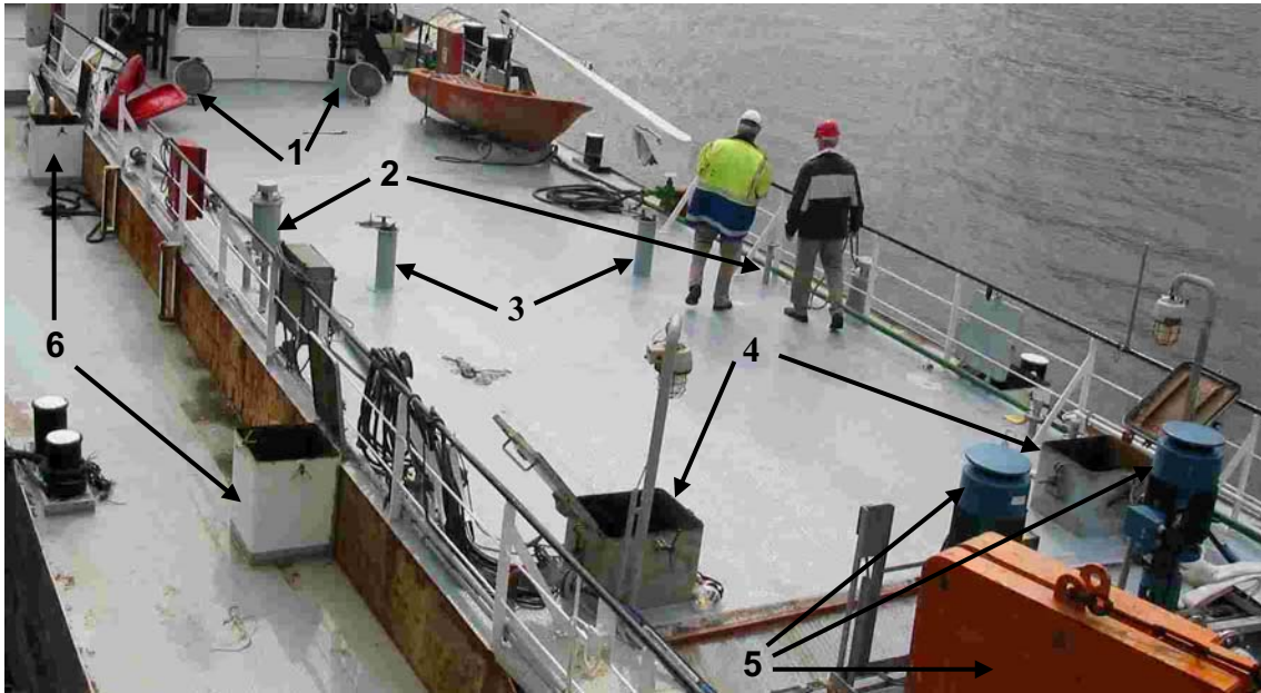
Figure 8: Tank apertures ENA 2 21
