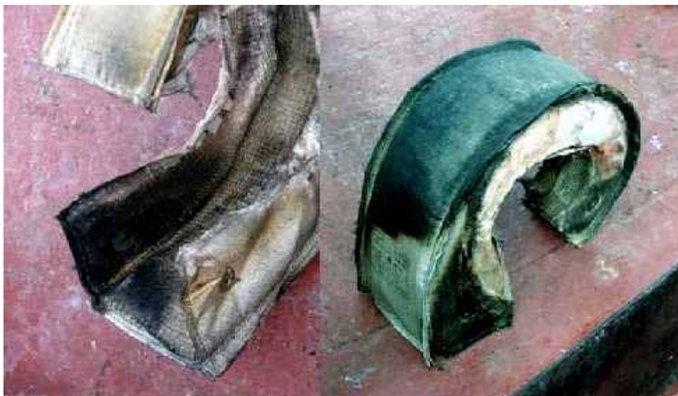
Figure 17: Insulation exhaust gas turbocharger
