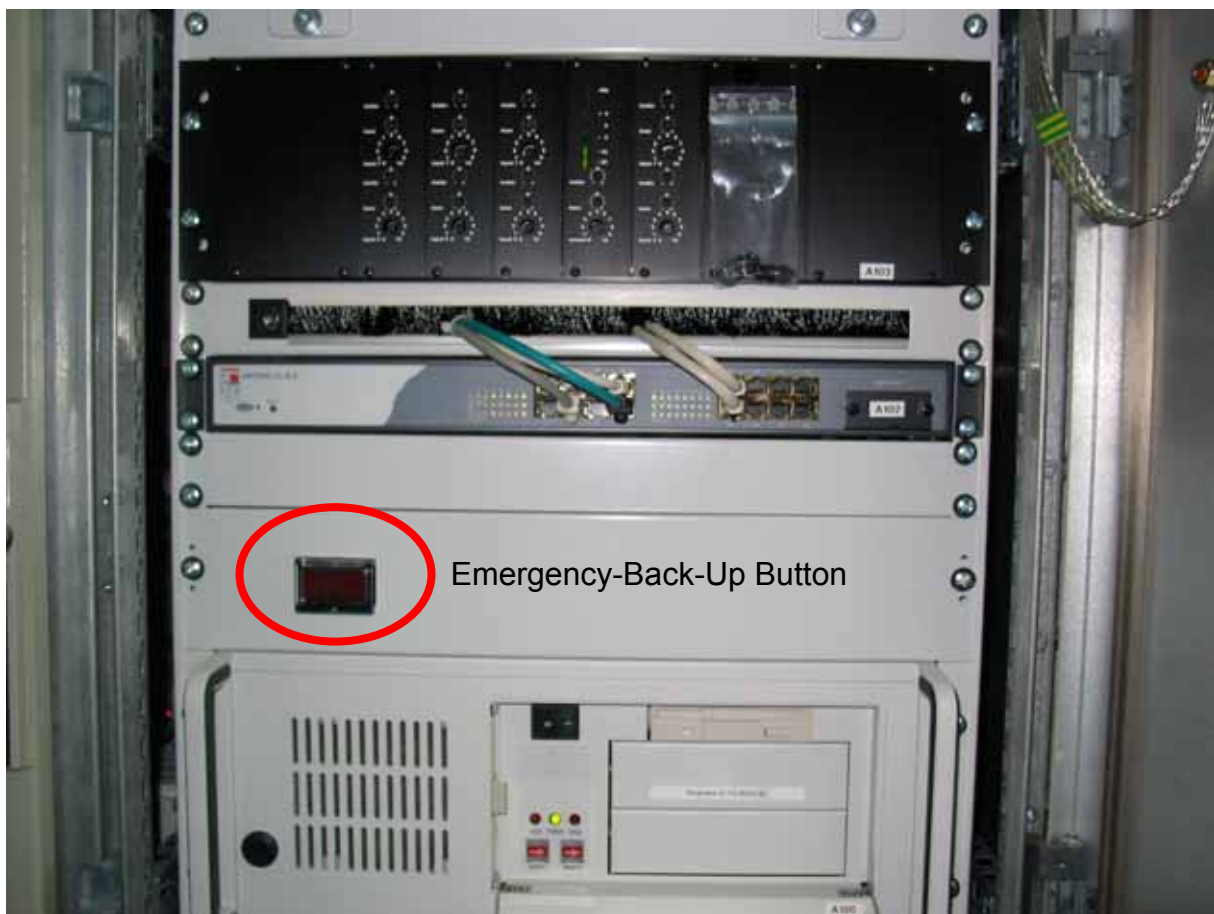
Figure 7: Emergency-Back-Up-Button on the VDR (Photo: Federal Bureau of Maritime Casualty Investigation)
