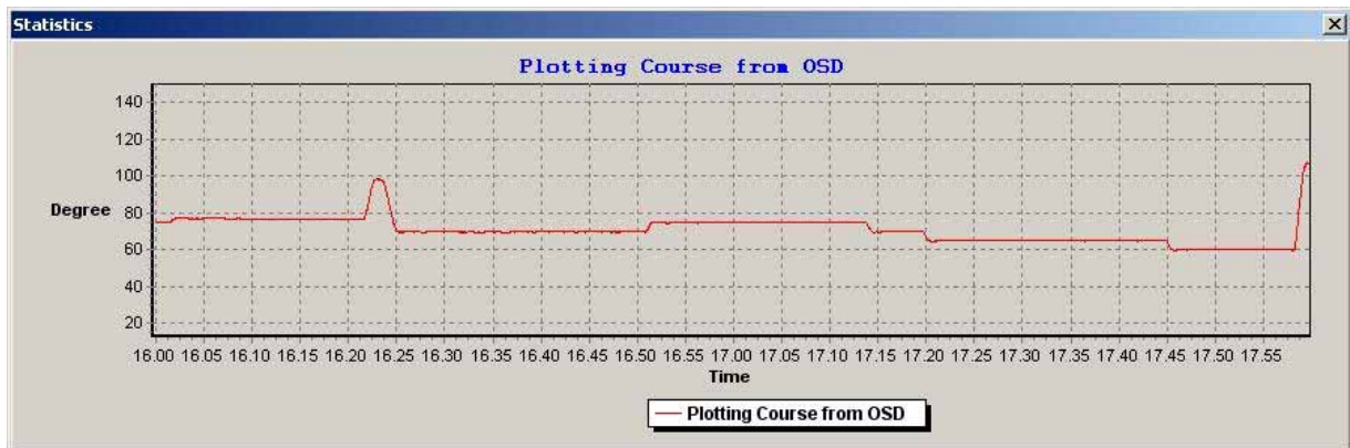
Figure 8: Changes of course of RITHI BHUM between midnight and 02:00 h on 14.11.2004 (Print from VDR RITHI BHUM, times UTC)
