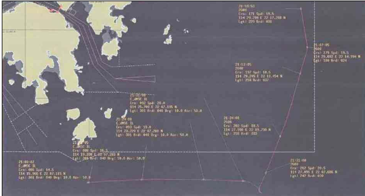
Figure 6: Radar plot of Radar Station Hong Kong at 21:00 h [at the lower image edge MSC ILONA on an easterly course, on the right HYUNDAI ADVANCE on a south/south-westerly course] (Source: Marine Department Hong Kong)
