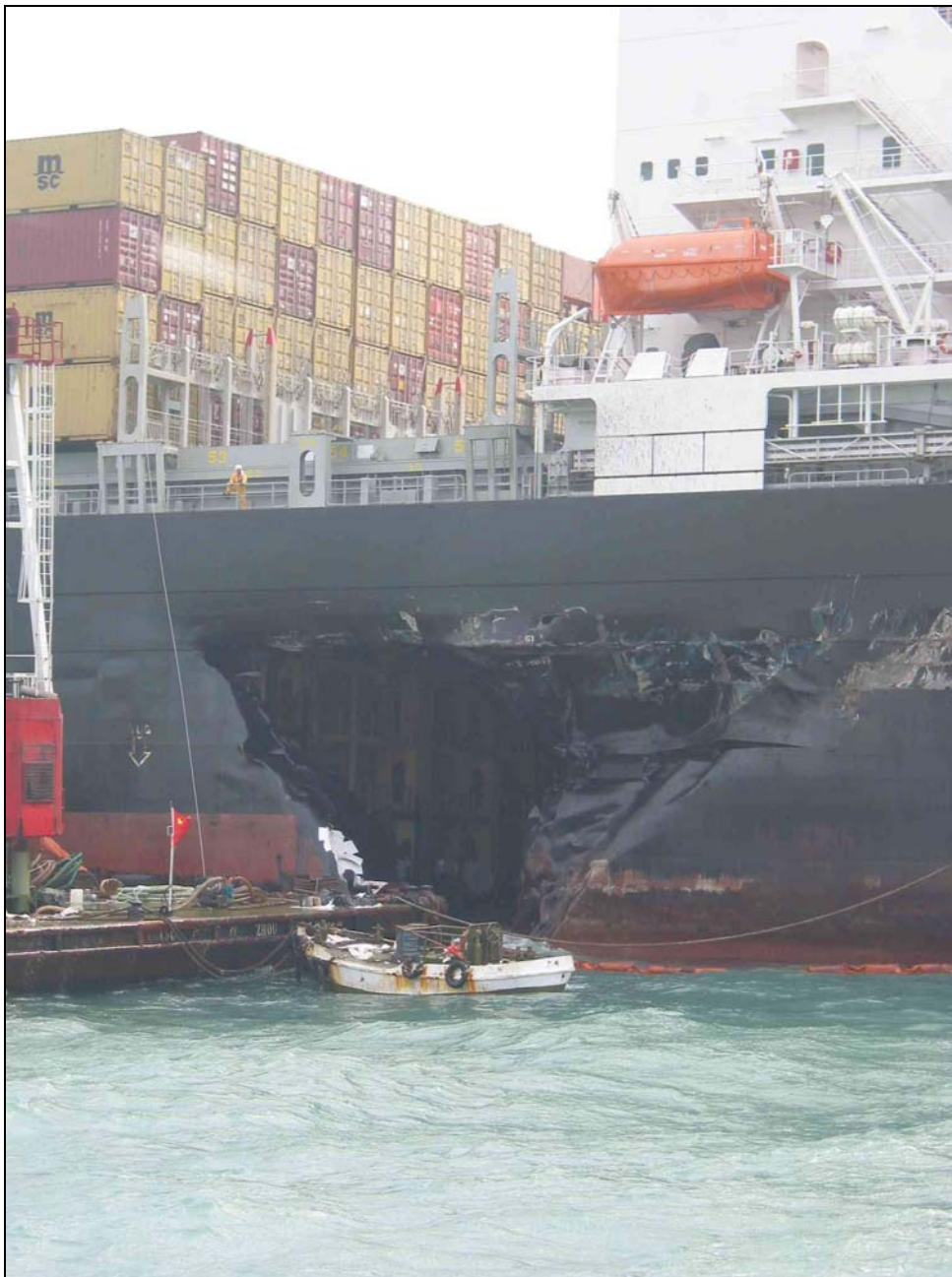
Figure 10: Damage to MSC ILONA (Photo: BSU)
