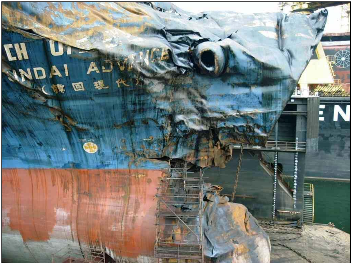
Figure 9: Damage to HYUNDAI ADVANCE (Photo: Korean Maritime Safety Tribunal)
