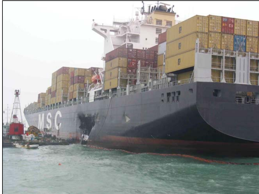
Figure 2: MSC ILONA (at the allocated anchor position after the collision, photo BSU)
