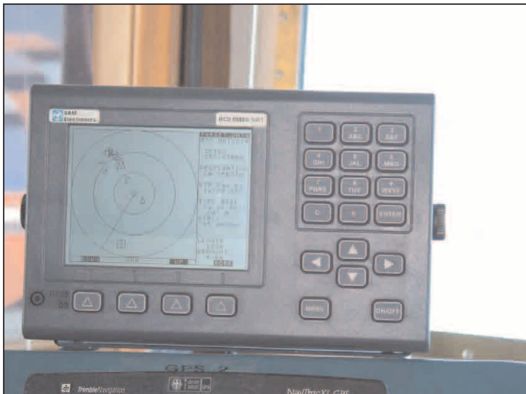
Photograph of the AIS on board Washington Senator
