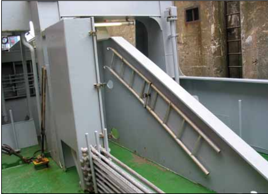
Figure 9: Example of a stored ladder (sister vessel)
