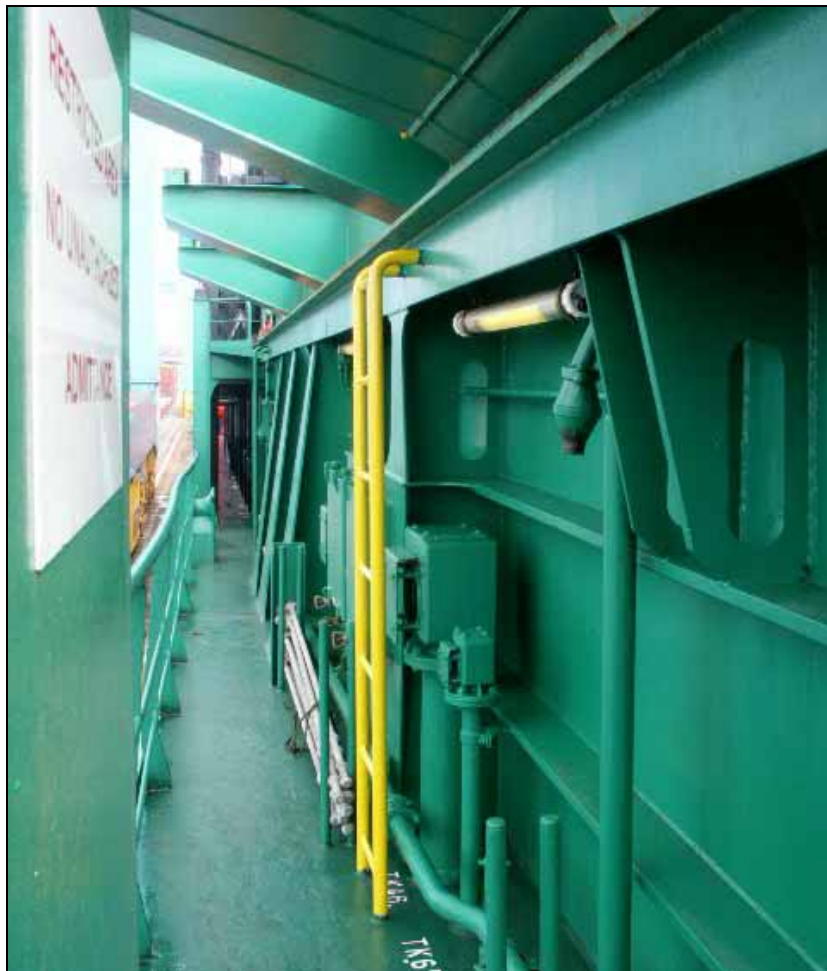
Figure 6: Ascent facility to hatch 2 (without ladder at the time of the accident)
