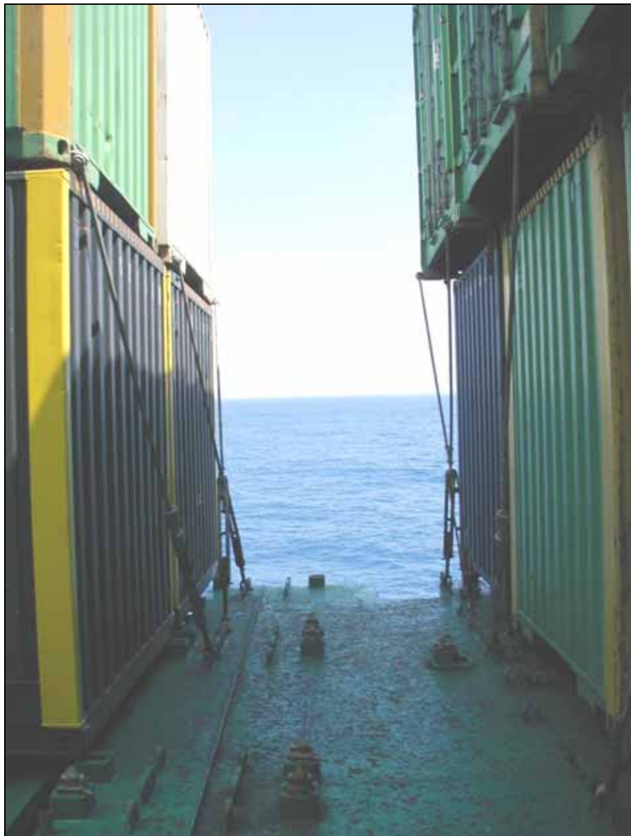
Figure 7: Loading situation after the accident in the lashing passage on hatch 2
