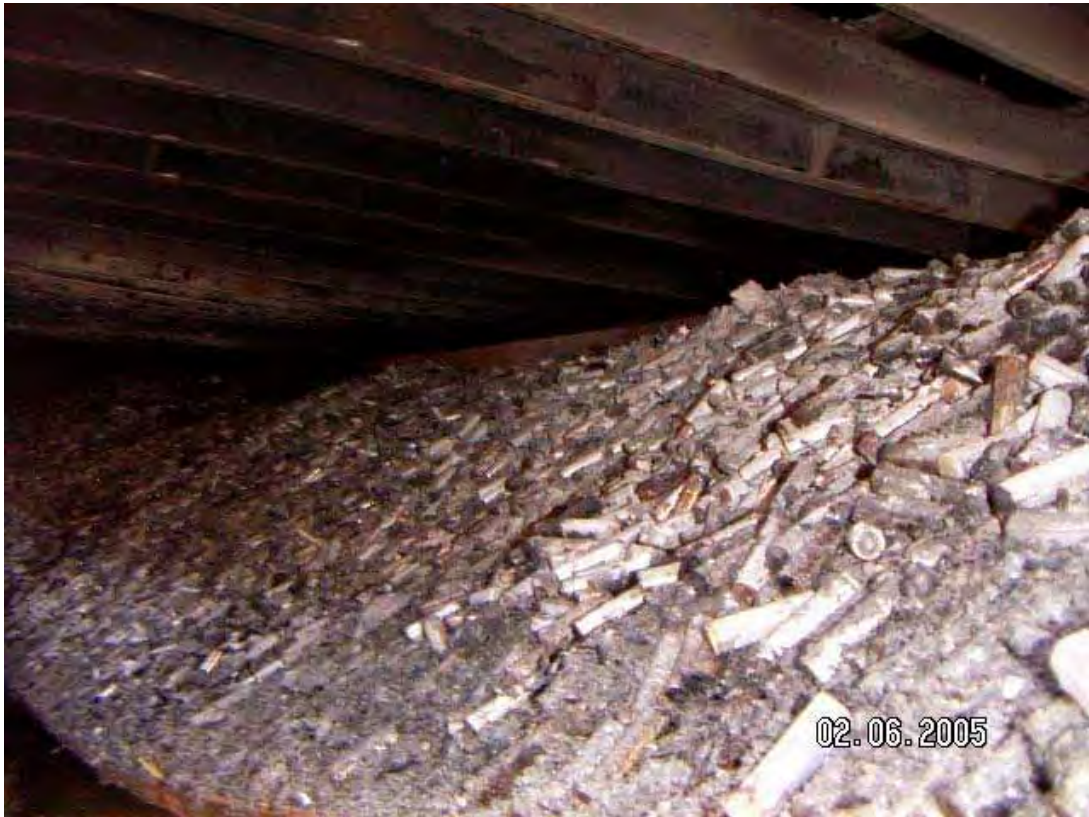
Figure 14: NiMH rechargeable batteries after the fire
