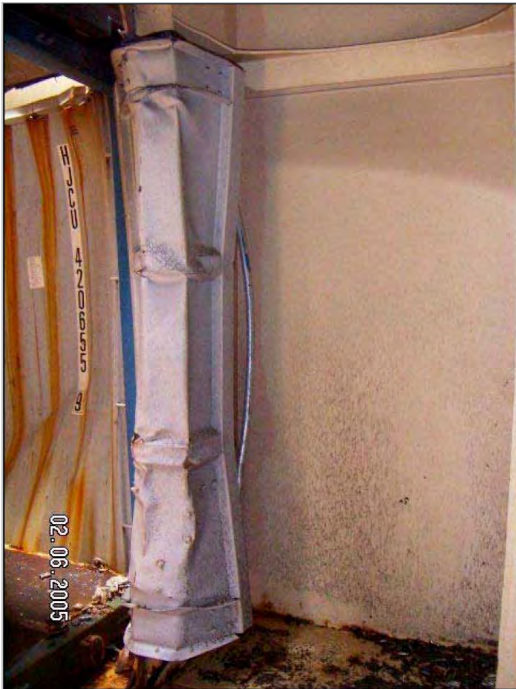
Figure 9: Container door of Container 1 wrapped round the frame
