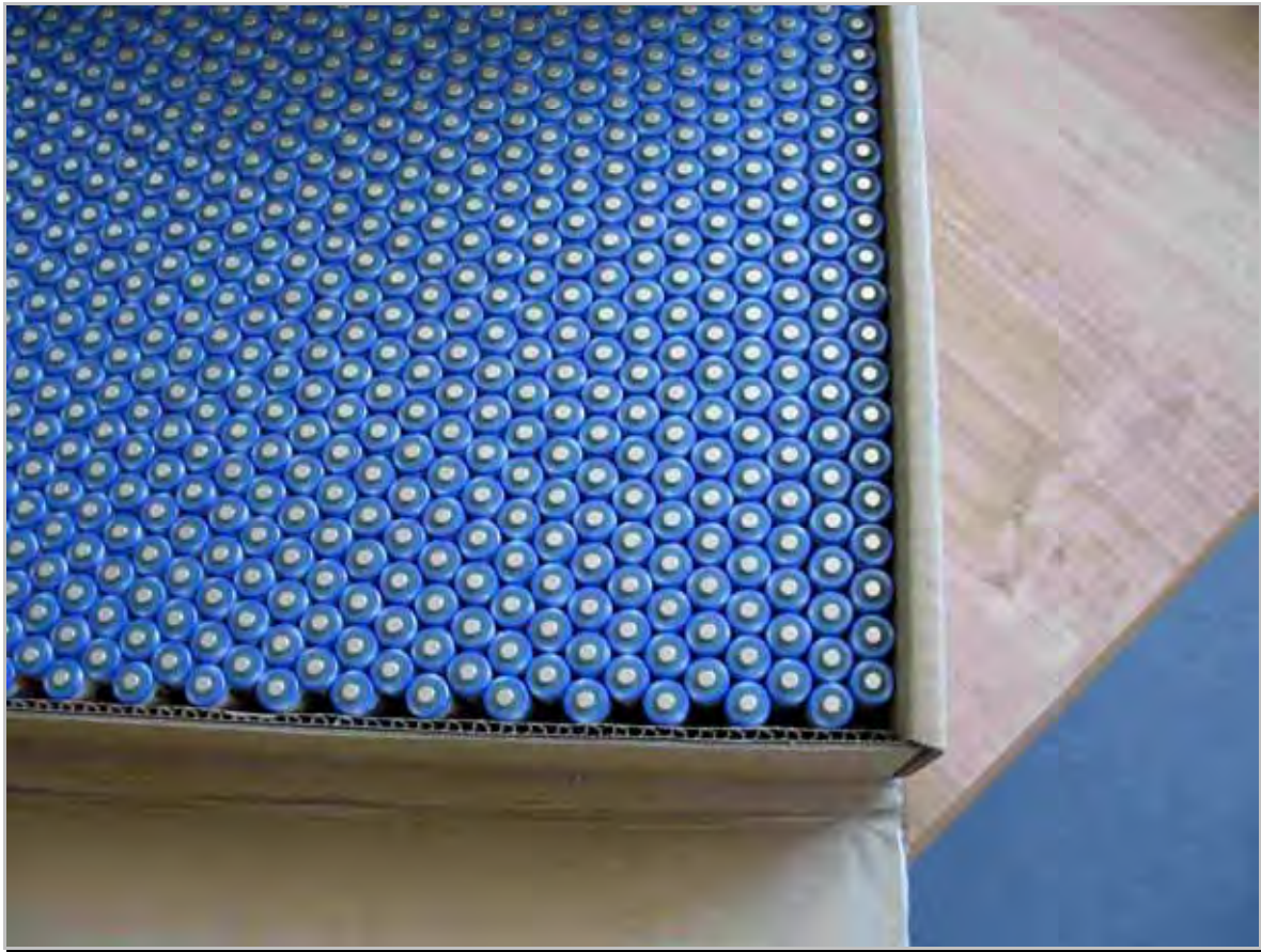
Figure 25: Rechargeable batteries, stored upright
