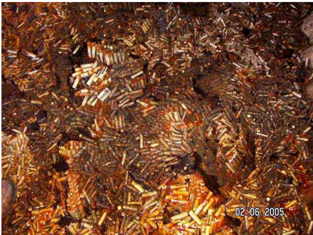
Figure 15: NiMH rechargeable batteries after the fire
