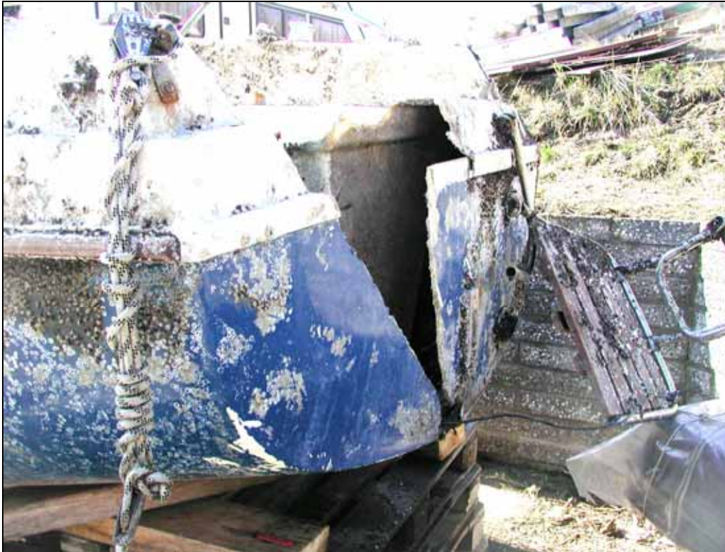
Figure 7: Straight cut edges at stern
