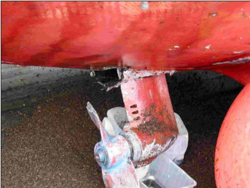
Figure 9: Saildrive shaft pushed forward and damaged propeller
