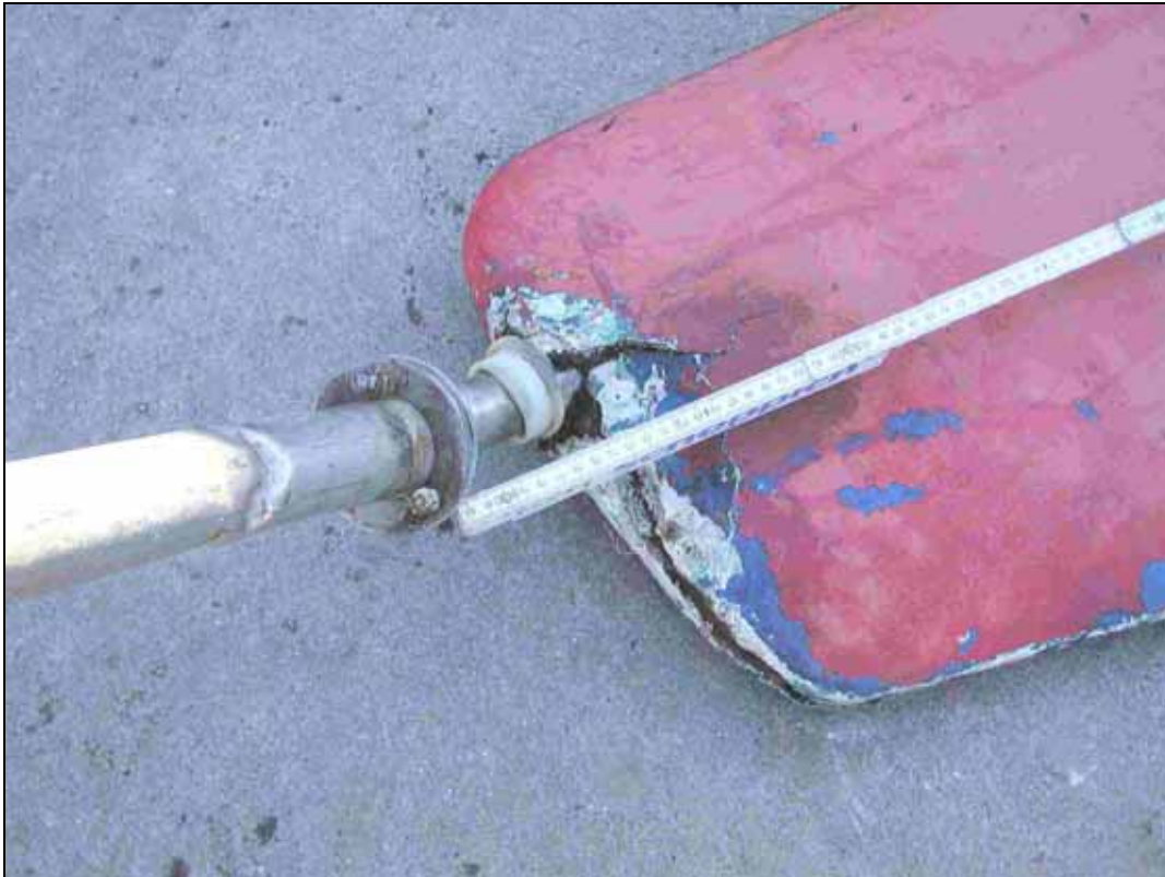
Figure 11: Upper part of the rudder blade with buckling
