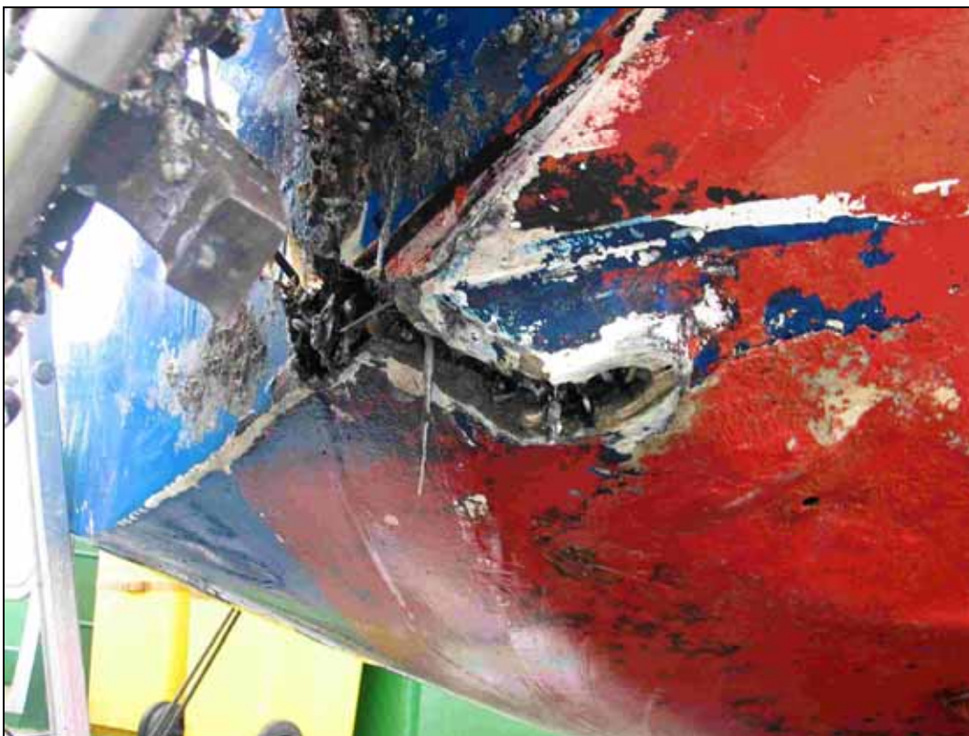
Figure 8: Crack in the bottom
