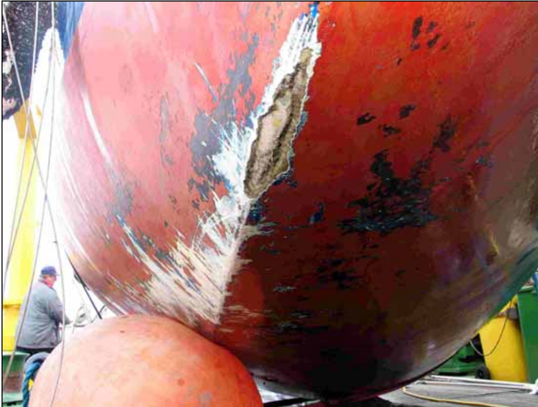
Figure 13: Damage to the bow
