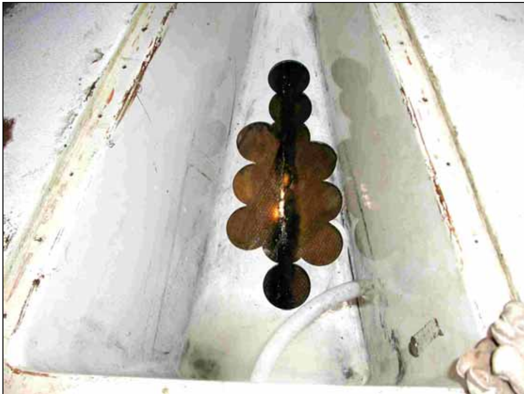
Figure 15: Inner shell cut open in the fore ship
