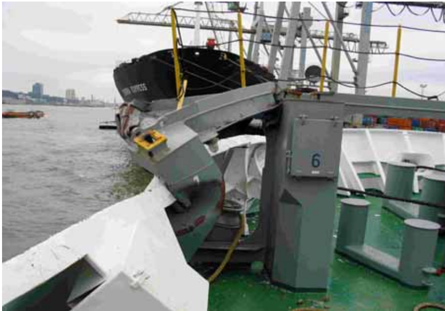
Figure 9: Damage to NEDLLOYD FINLAND (2)
