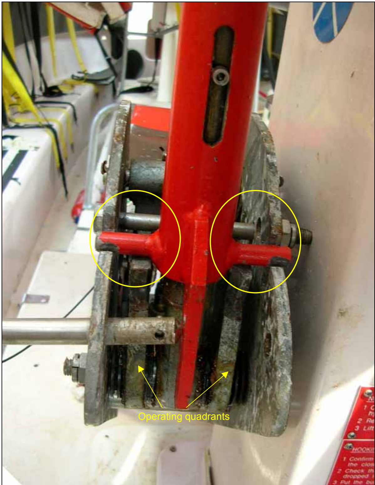
Figure 11: Release unit after the accident; the leading pins resting on the operating quadrants
