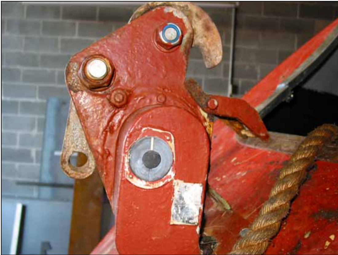
Figure 14: Forward releasing hook, port side, with red and white sector lacking on the cover
