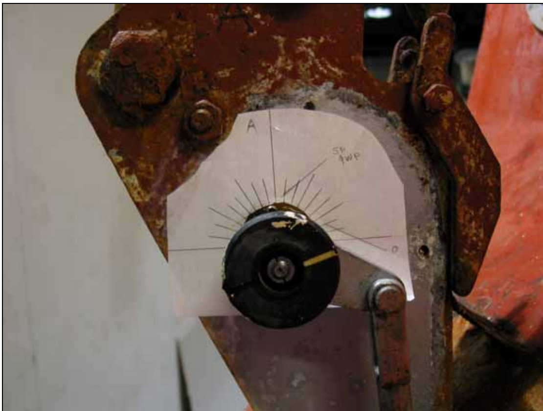
Figure 17: Aft releasing hook with graphometer and recorded angles
