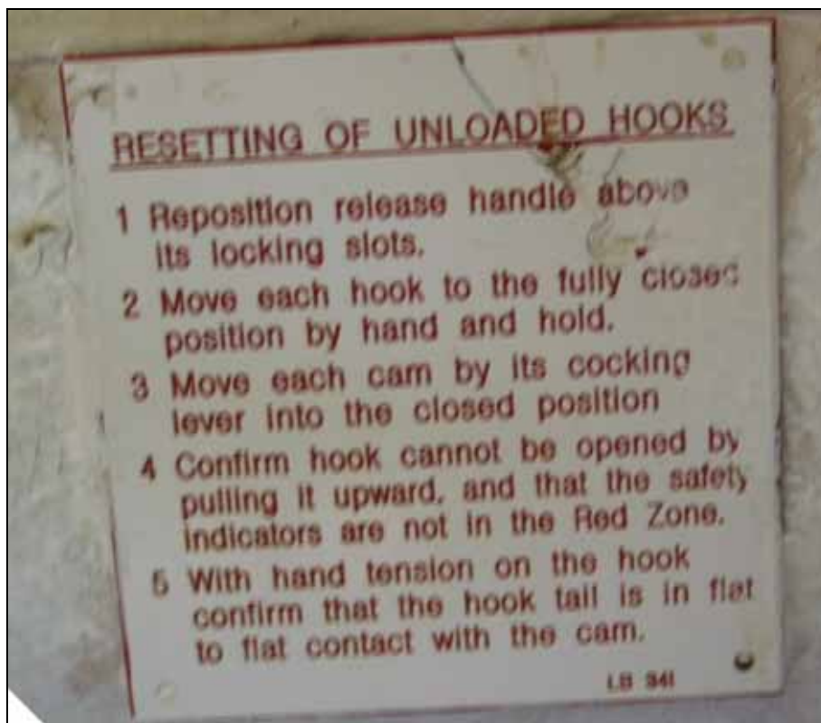
Figure 18: Description of the handling of the releasing hooks, plate LB 34i
