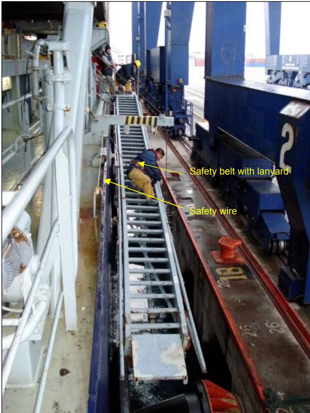
Figure 4: Unfolded gangway with safety wire 4
