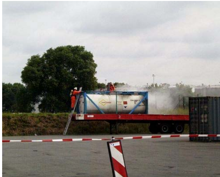
Fig. 8: Operation using protective clothing and breathing apparatus
