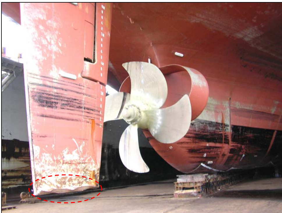
Fig. 6: Deformations on the rudder blade 23
