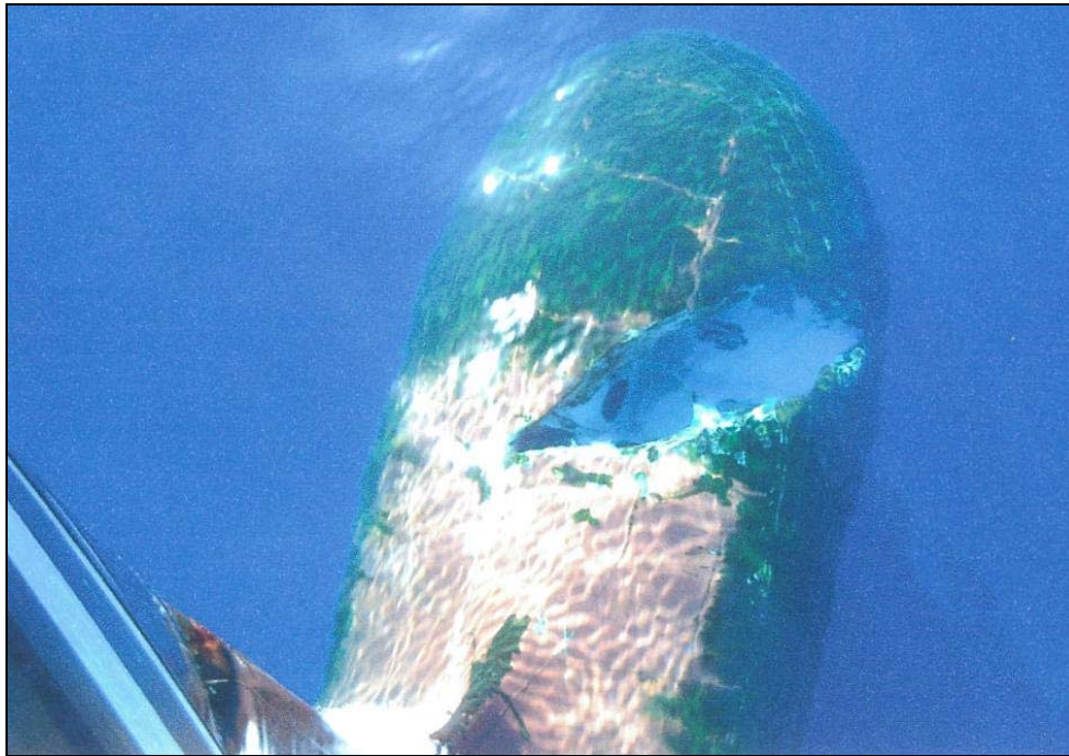
Figure 8: Damage on the bulbous bow of HANJIN CAIRO
