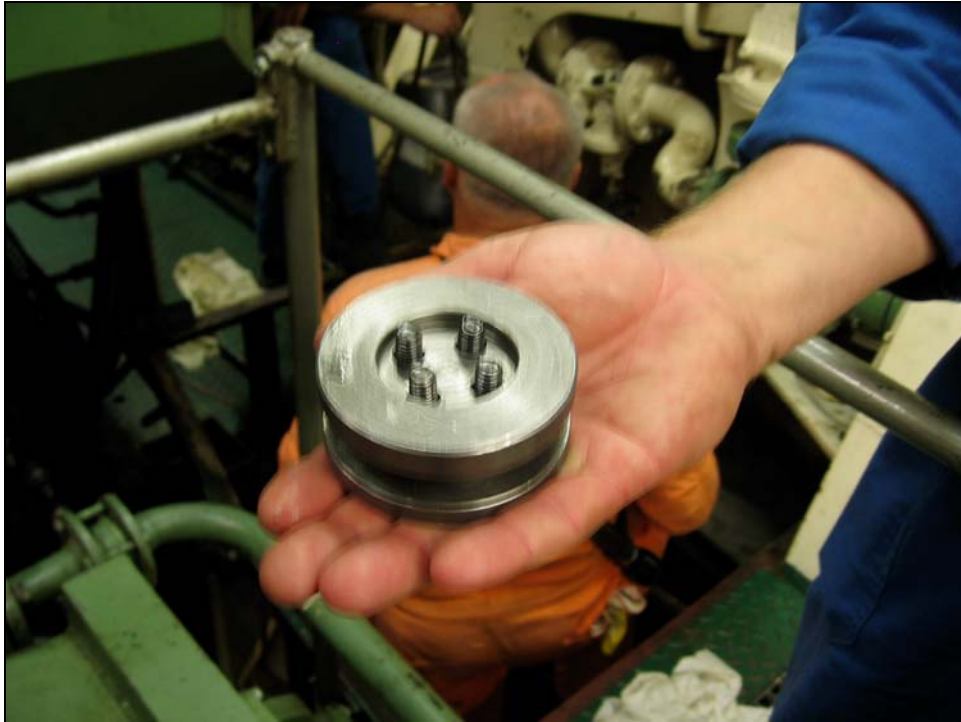
Figure 11: Demounted double sheave from the OD box
