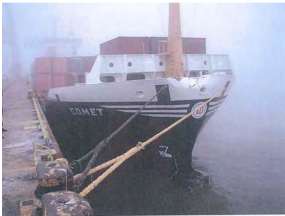
Fig. 4: Bow damage COMET
