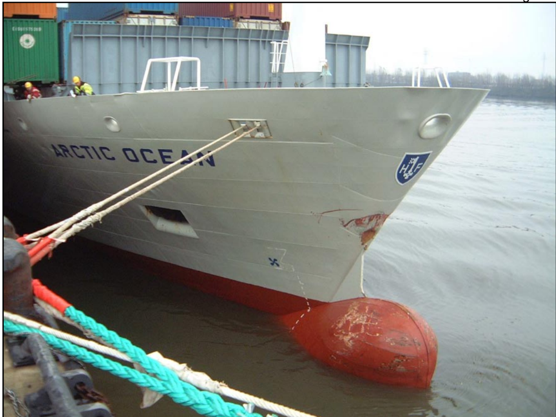
Damage to bows of Arctic Ocean
