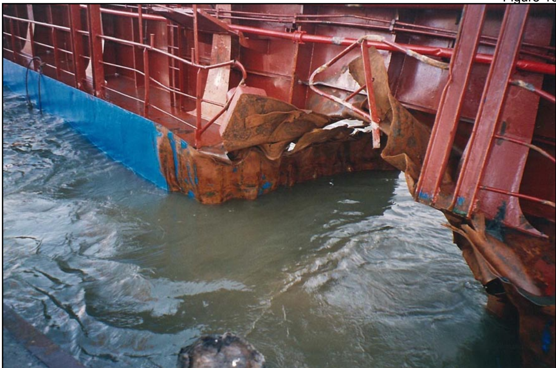
Damage to starboard side of Maritime Lady
