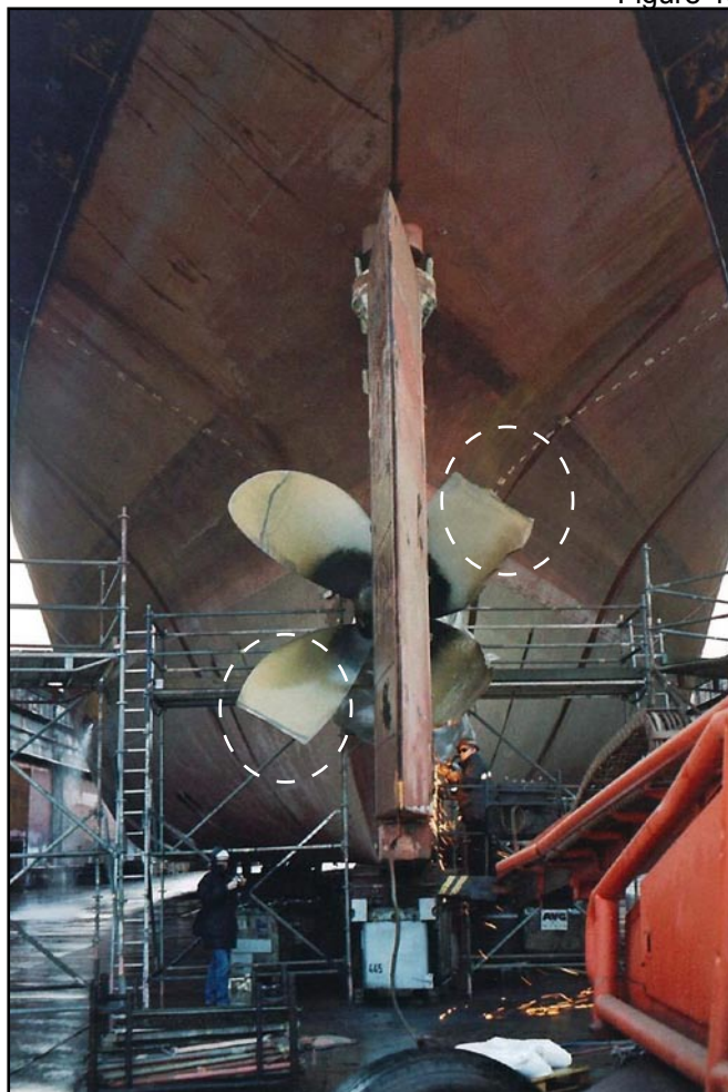
Propeller of Sunny Blossom - showing two cropped blades
