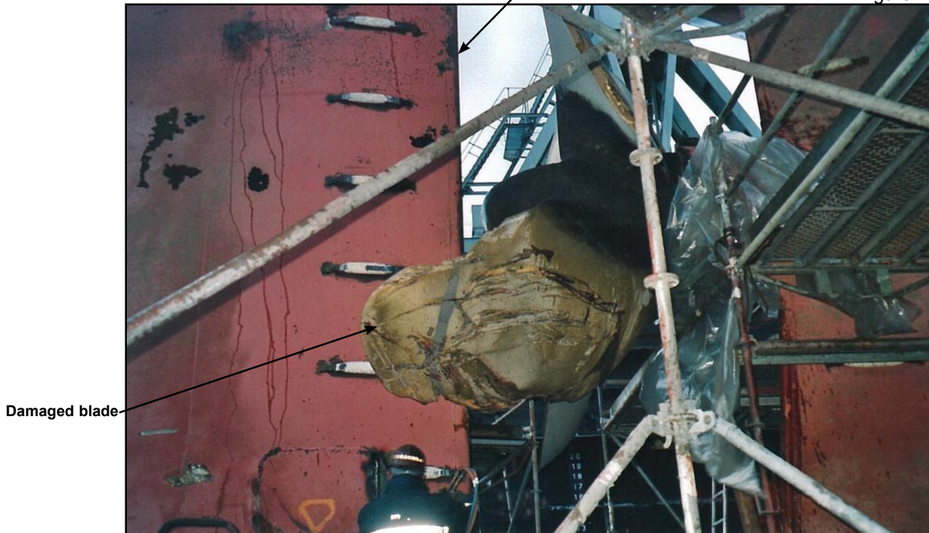
Damage to propeller blade of Sunny Blossom
