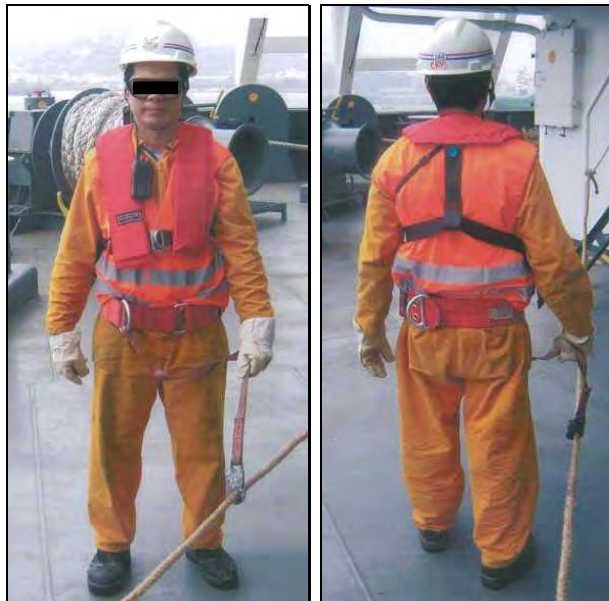
Figure 8: Full personal protection equipment as intended to be worn for work on deck
