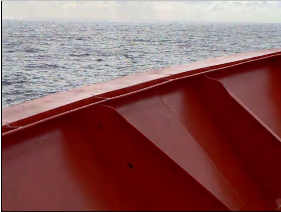
Figure 15: Additional rail installed on board the CAP EGMONT
