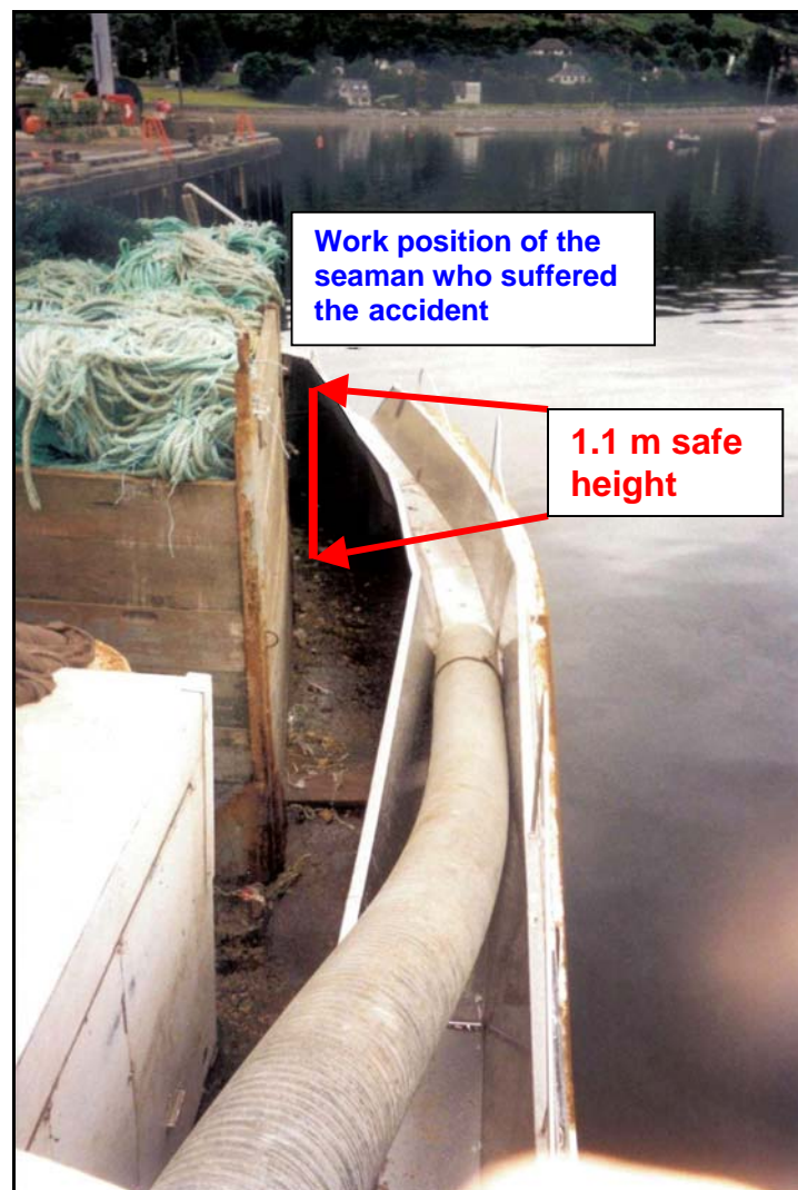
Figure 7: FV BELEN – Channel for launching the net
