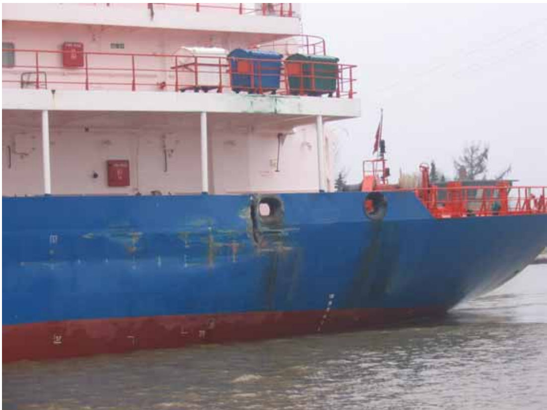
Figure 18. Damages on the side of the WOLGASTERN. (the picture on behalf of BSU)
