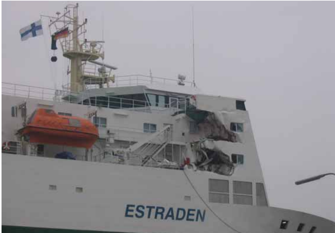
Figure 13. Damages of the ESTRADEN's SB-side. (the picture on behalf of BSU)
