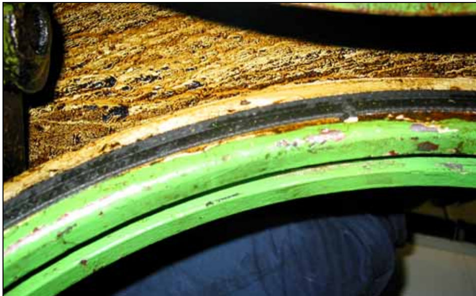
Figure 28: Gasket glued onto the hatch frame
