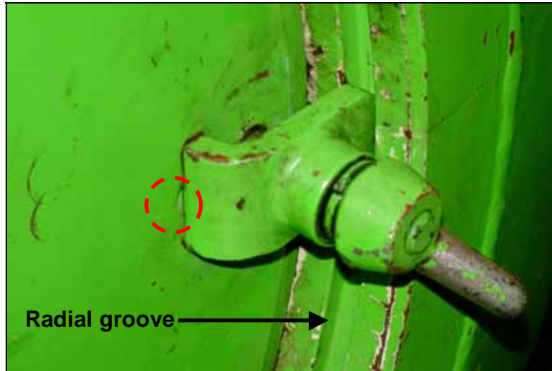
Figure 27: Bolt swung into the full locking position
