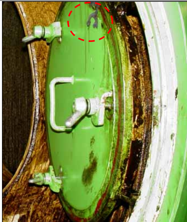
Figure 49: Remains of the jammed object – overall view
