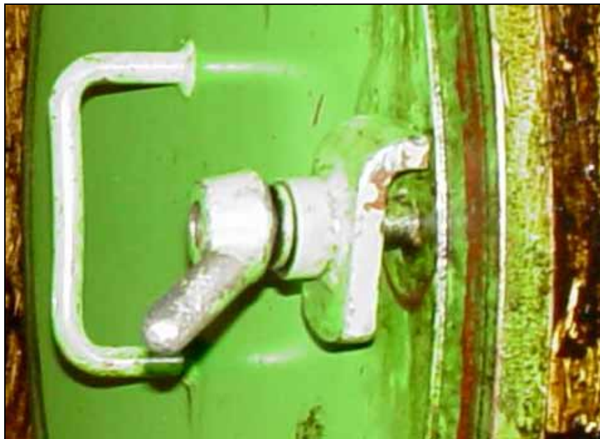
Figure 26: Bolt in open position (L-profile visible)
