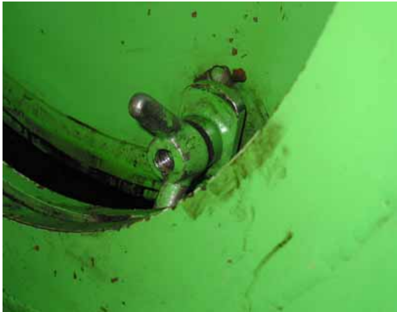
Figure 32: Double wing toggle nut as a blocking obstacle
