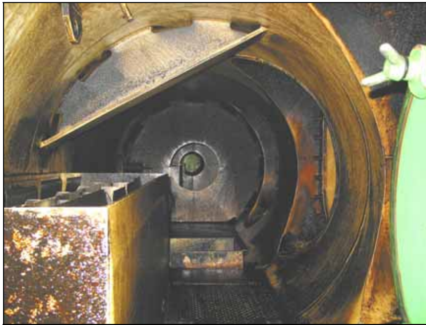
Figure 44: View from the forward end into the scavenge air receiver, with aft hatch open
