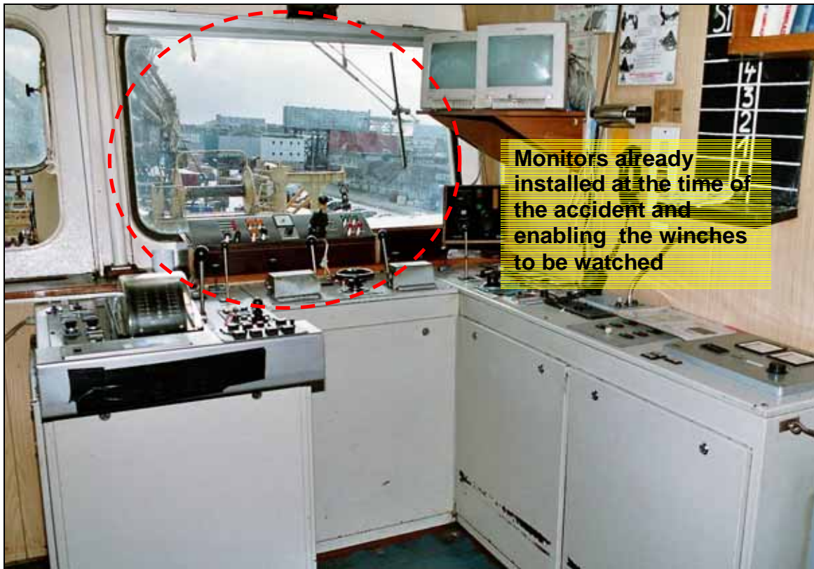
Figure 15: Winch operation control position with bridge windows
