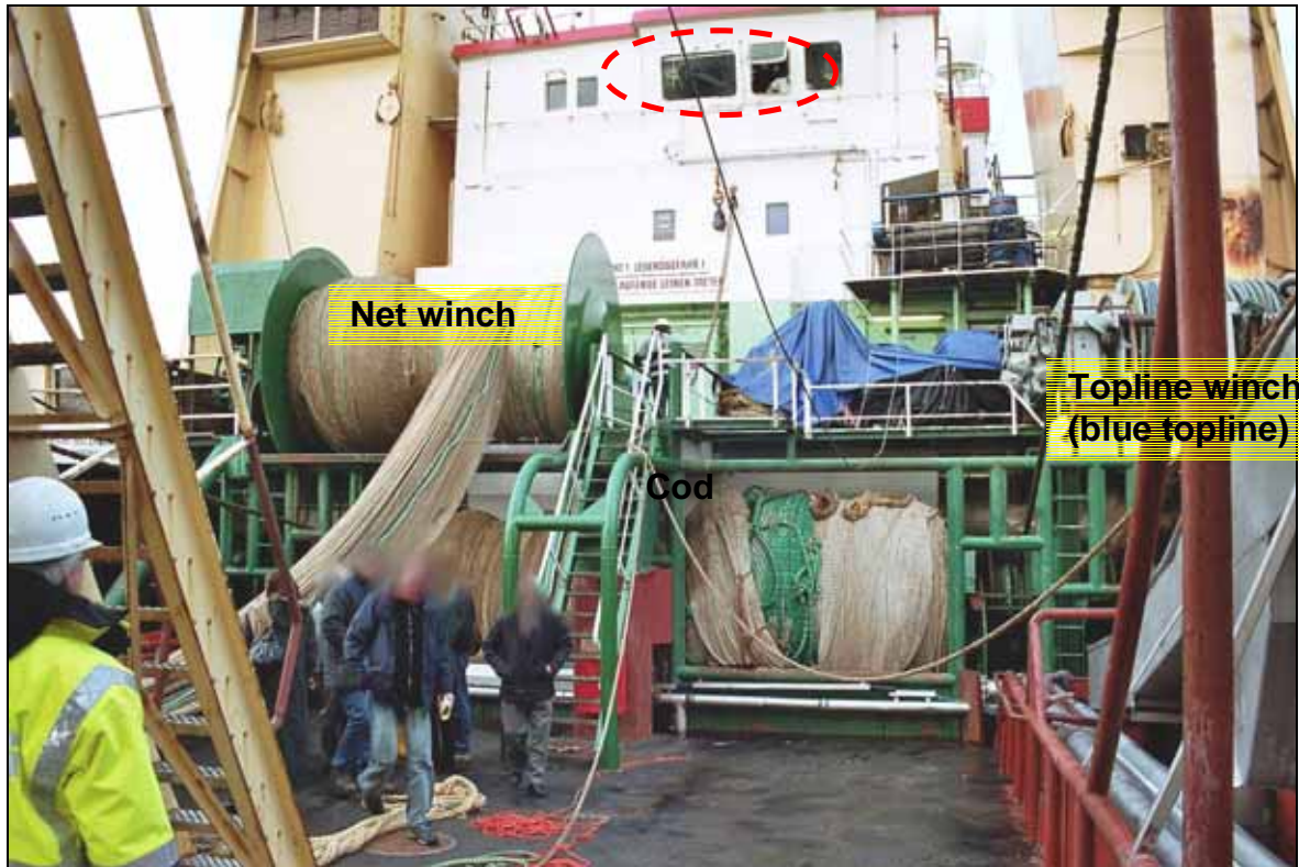
Figure 9: View from the fishing deck towards the after edge of the bridge 9
