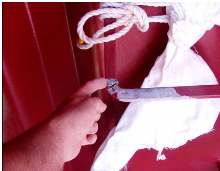
Figure 9: Broken ladder rung
