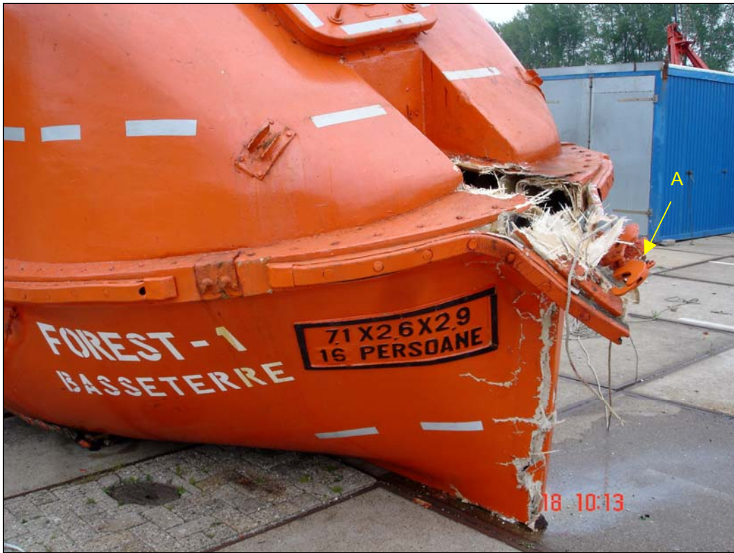
Figure 11: Damage to the bow due to releasing hook having been torn out; A = hook for forward painter
