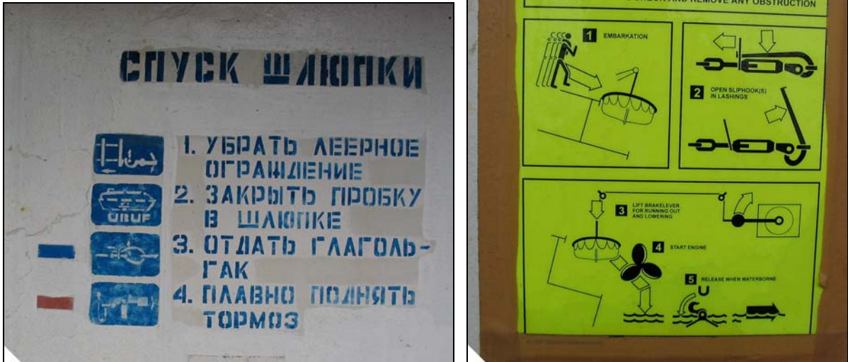
Figure 3: Description of the launching procedure in Russian and English, posted on the boat deck
