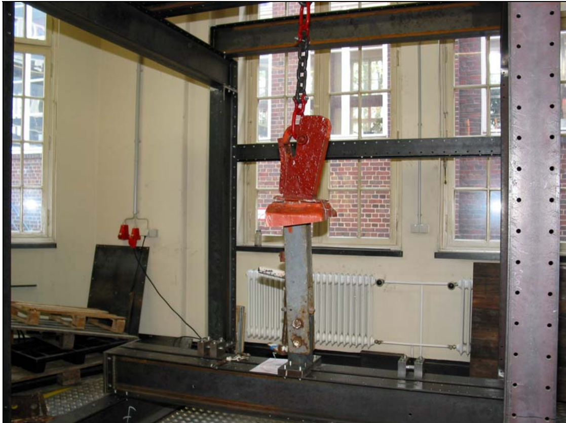
Figure 20: Test frame with aft releasing hook (lateral view)
