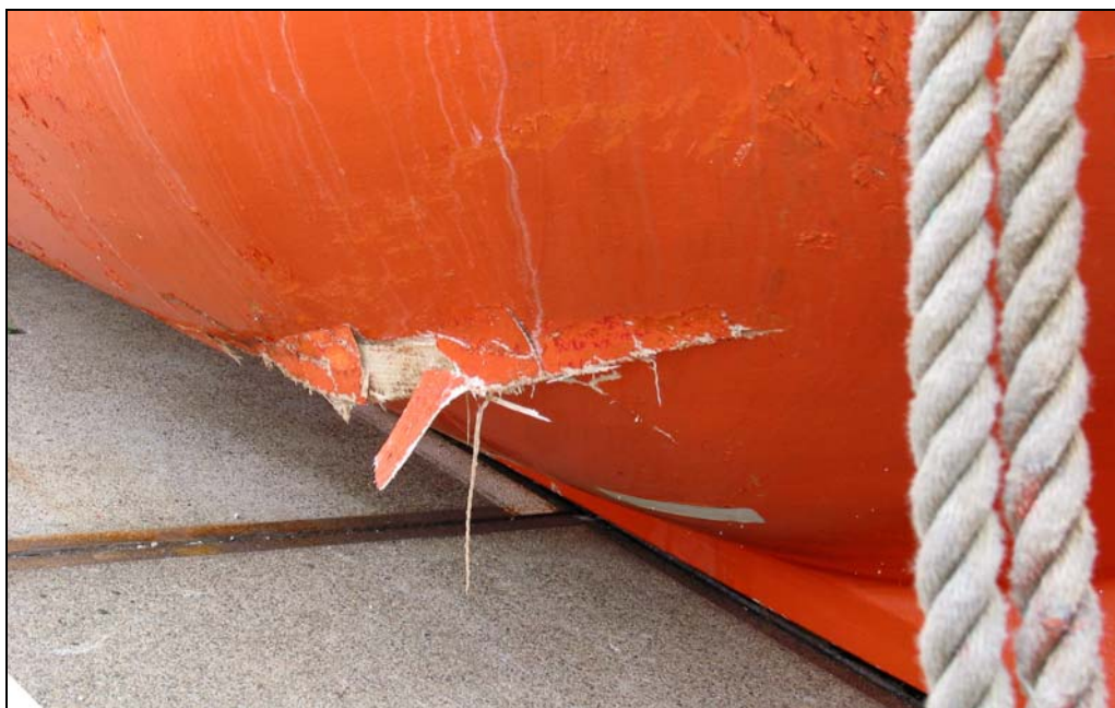
Figure 10: Hull broken open on the port side aft
