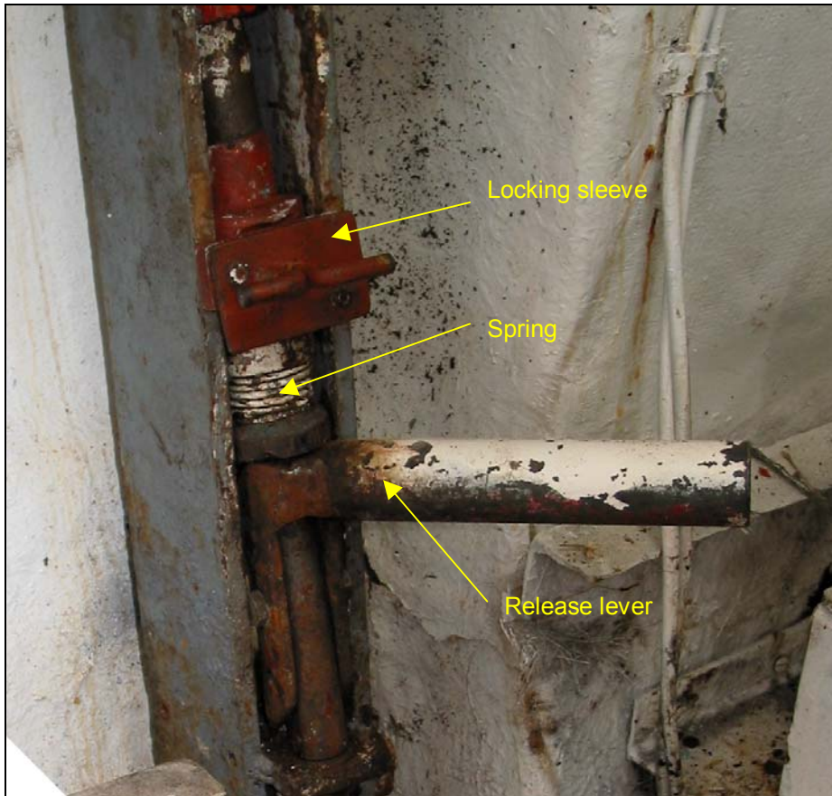
Figure 16: Aft release unit; release lever raised, spring under tension
